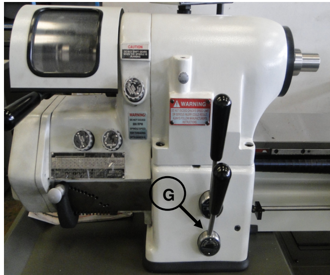
Figure 10-Control Speed and Direction
