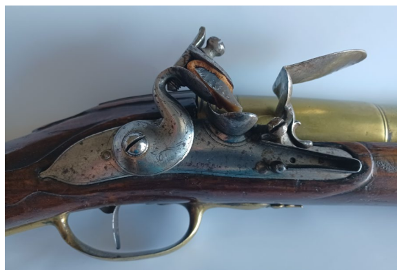
Figure 1. Bleiberg lockplate with BLEIBERG at bottom in front of the hammer.
