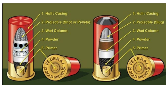
Figure 113. Diagram of a shotgun shell cartridge (Instructables Craft 2022).
