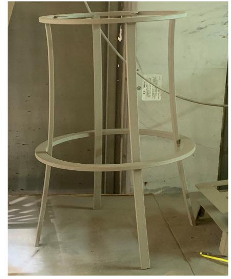
This is my design and production of a full scale bar stool to be completed with upholstered seat. Fabricated from shop found scrap and completed through powder coating. Also shown is the "scaffolding" used as I ensured the chair came out square.
