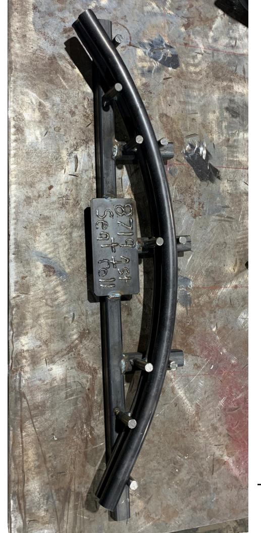
This jig was created to ensure a specific piece of a specific bar stool in the J.C. catalogue is always bent to the right degree. This jig is and will remain part of the commercial mass production of this stool.
