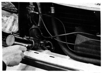
Use a leak detector to check all connections.
