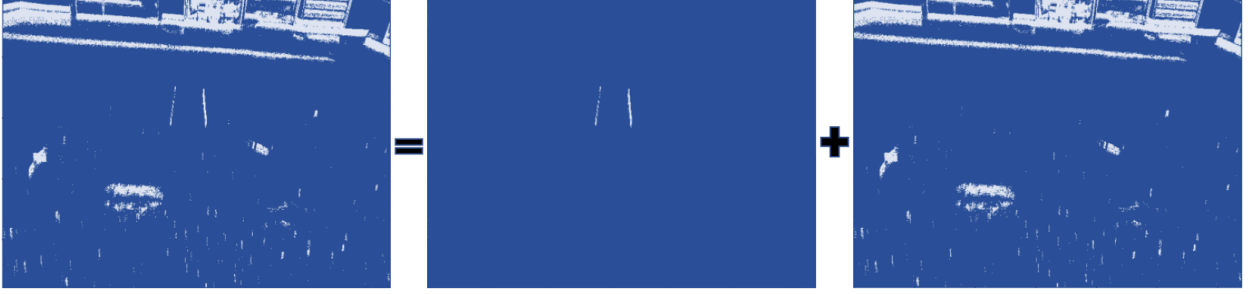
Figure 3.2: Monochromatic images generated using state-of-the-art event-based cameras. The full image I to the left can be decomposed into one that contains only the runway image I_r (center) and the remaining objects/noise I_n (right), i.e., I = I_r + I_n .
