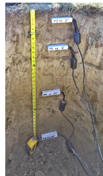
Figure 3: Soil pit in silty loam near Roundup, MT. The probes record changes in plant available water, temperature, and soil water quality.
