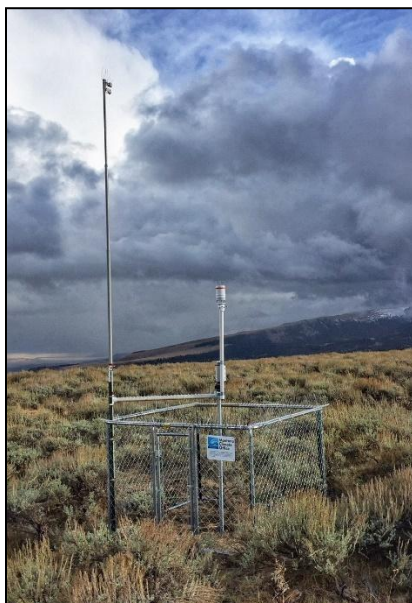
Figure 2: Completed station in sagebrush rangeland west of Dillon, MT with optional NDVI sensor pair measuring vegetation greenness. NDVI can be used to track vegetation health and forage production.
