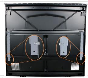
14. Place  $5/16-18 \times 1/2$ " Button head bolt thru the Hood Support and the hole. Then from inside the hood cross brace place a flatwasher and 5/16-18 Locknut and tighten. (repeat on Driver's side)
