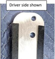
5. Using the supplied hex key, bolt the Bow Mount (B2) with the <u>tall</u> section of (B2) facing towards the front of the Bronco to the top of the Bedside Mount with (4) black ¼-28 x 3/8" button head screws. Use blue Loctite (not included).
