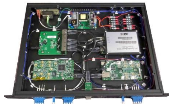
1U chassis with multiple custom PCBs installed and Ethernet control interface
