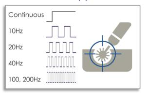
Not only continuous mode but also pulse mode supports for more precise control as similar with CO2 laser equipment
