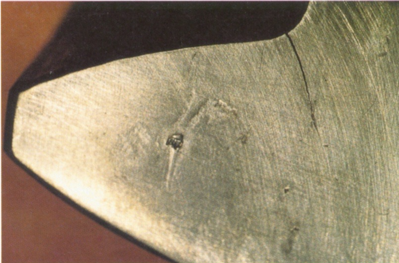
Bending fatigue crack
