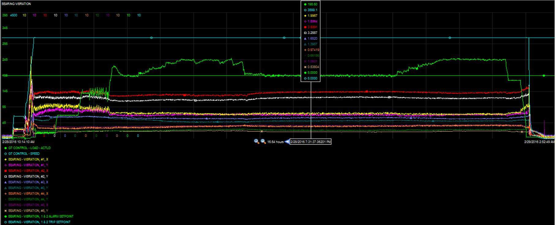
Overall Vibration levels after balancing was performed by installing trim balance weights in the turbine end of the machine.
