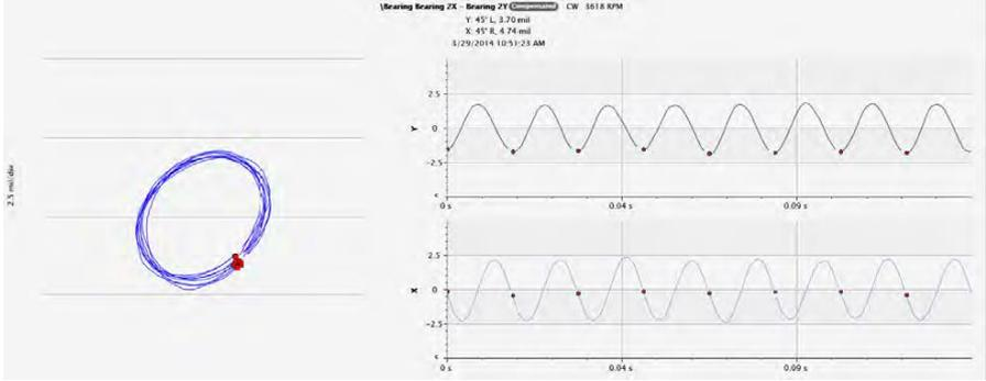
Startup and initial loaded operation; clean 2<sup>nd</sup> critical; but some vertical preload as it reached full speed - #2 bearing on the same machine.
