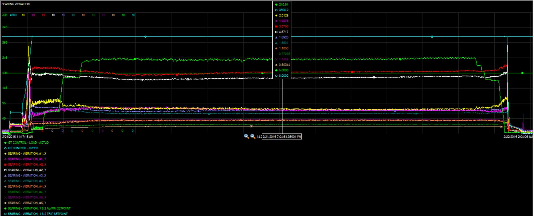
Overall Vibration levels after a row 2 turbine blade replacement. Note blades were changed on turbine end, higher vibration incurred on compressor end.
