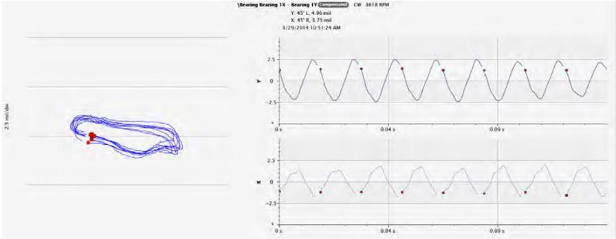
Startup and initial loaded operation; clean 2<sup>nd</sup> critical; but some vertical preload as it reached full speed; #1 bearing
