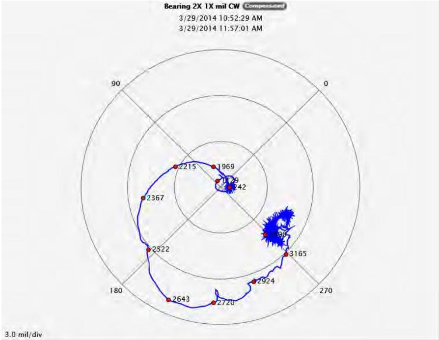
Polar plots – Bearing 1 on the left; bearing 2 on the right during coast down. Shows 180 degree phase shift between ends at the 2<sup>nd</sup> critical.
