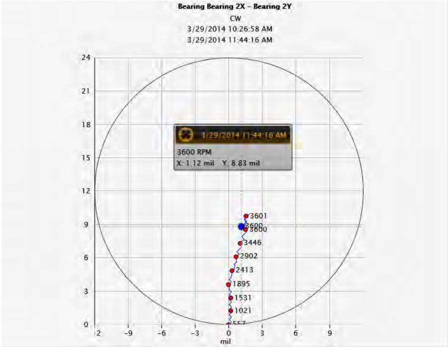
Shaft Centerlines on the same machine during coast down. Rub on the #1 bearing was confirmed with the unusual shaft centerline movement.
