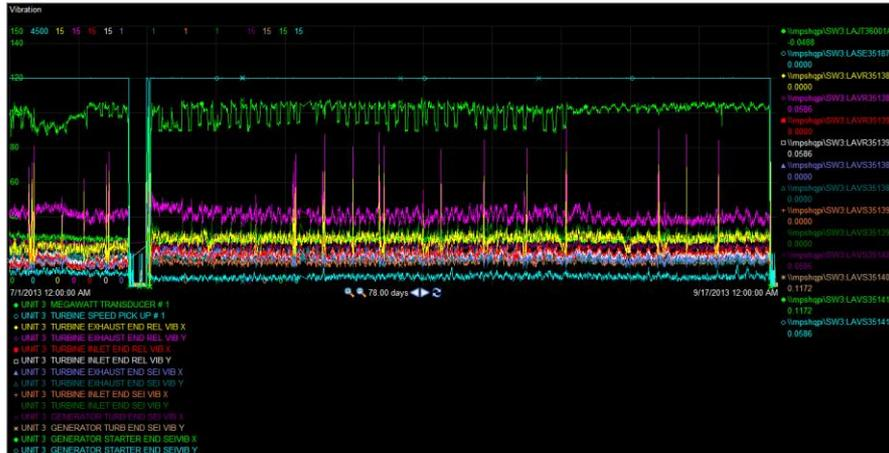
One amplitude increase was caught on dynamic data collection showing both amplitude swing and phase shifting
