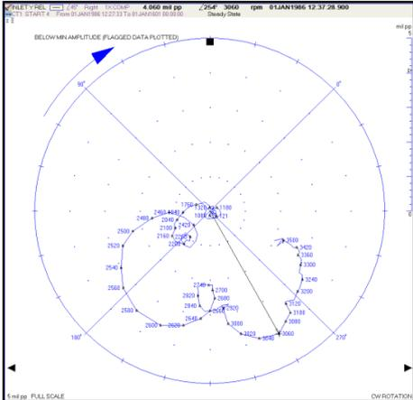
Polar plots showing 1<sup>st</sup> and 2<sup>nd</sup> critical responses and increased response after 2<sup>nd</sup> critical.
