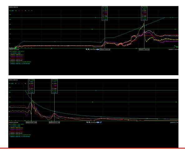
Startup and coast down overall trend behavior after trim balancing was performed by adding weights in the turbine end of the machine
