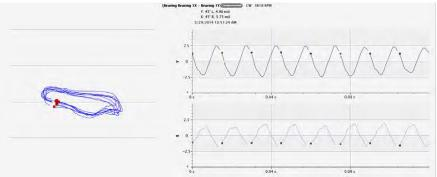
Startup and initial loaded operation; clean 2<sup>nd</sup> critical; but some vertical preload as it reached full speed; #1 bearing
