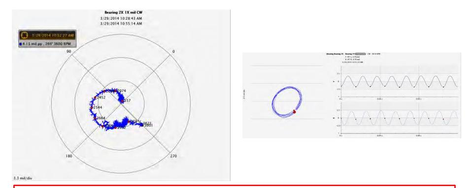
Startup and initial loaded operation; clean 2<sup>nd</sup> critical; but some vertical preload as it reached full speed - #2 bearing on the same machine.
