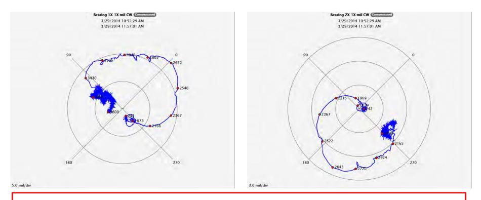
Polar plots – Bearing 1 on the left; bearing 2 on the right during coast down. Shows 180 degree phase shift between ends at the 2<sup>nd</sup> critical.
