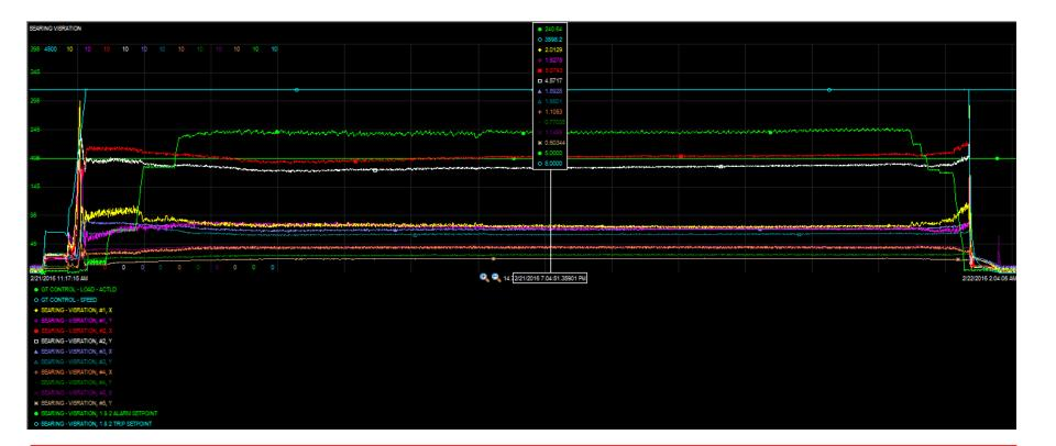
Overall Vibration levels after a row 2 turbine blade replacement. Note blades were changed on turbine end, higher vibration incurred on compressor end.
