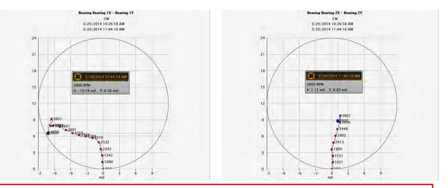
Shaft Centerlines on the same machine during coast down. Rub on the #1 bearing was confirmed with the unusual shaft centerline movement.
