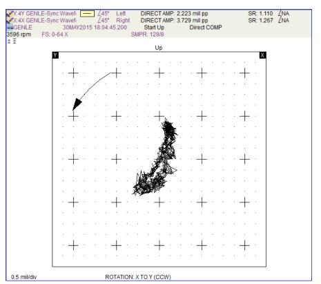
Example of a machine with preload on two of it's bearings looking at the Direct Orbits. Left side plot with banana shape; right side plot with 'flattened' side.
