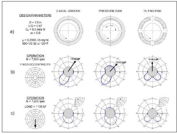
Know your bearings. Different bearings designs produce different operational characteristics.
