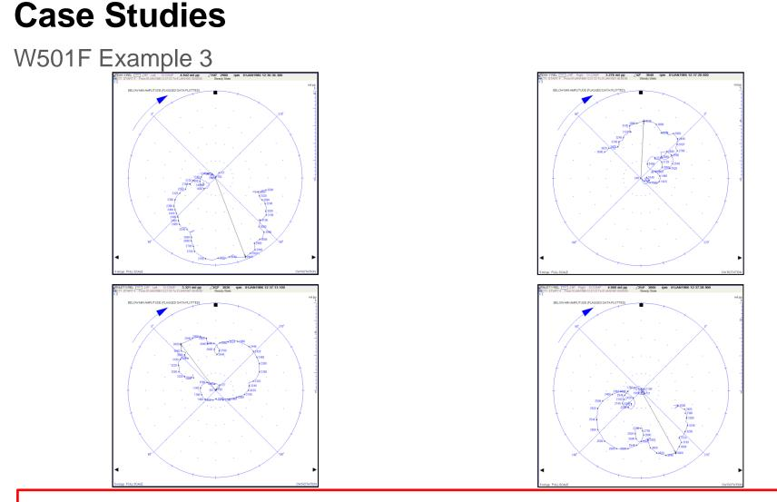
Polar plots showing 1<sup>st</sup> and 2<sup>nd</sup> critical responses and increased response after 2<sup>nd</sup> critical.
