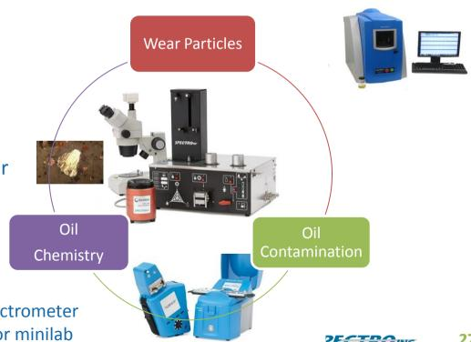
Walk-around portable viscometer and IR Spectrometer complements table-top Spectro 5200 Trivector minilab
