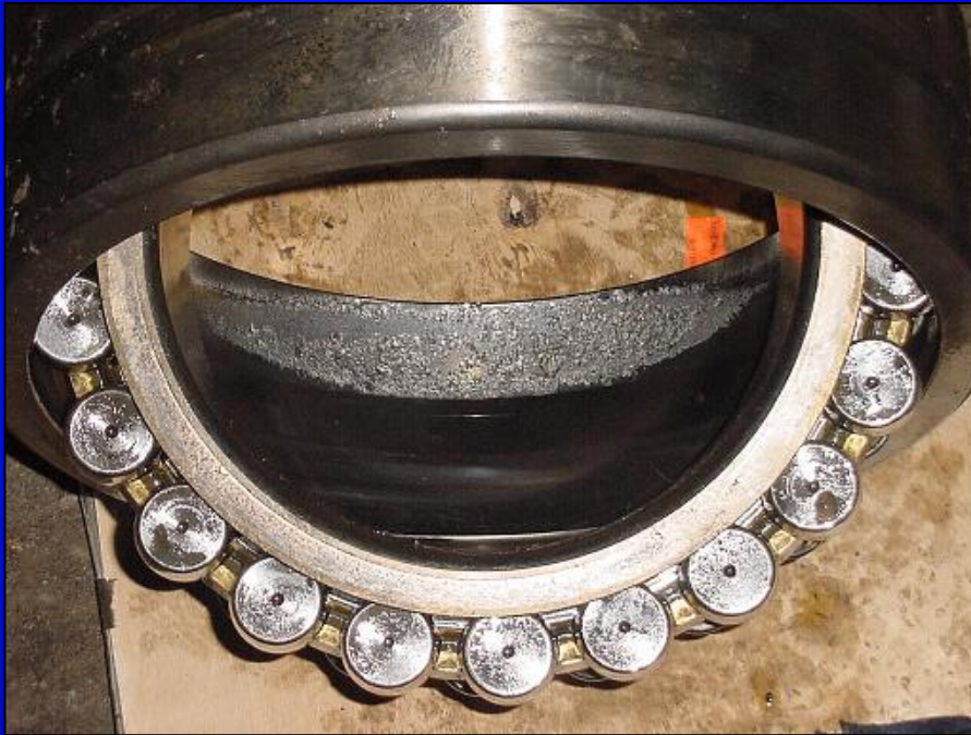
Outer race fault (spalling) on a spherical roller bearing.
