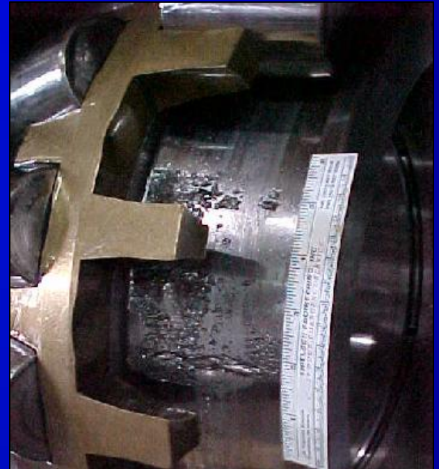
Inner race fault (spalling) on a triple race spherical roller bearing.
