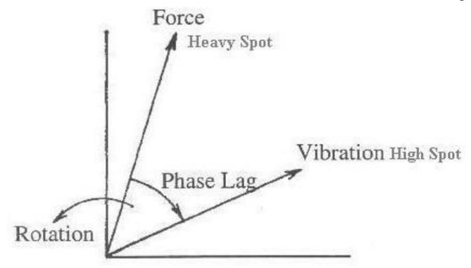
Initially the angular relationship of the Heavy Spot to the High Spot is unknown.
