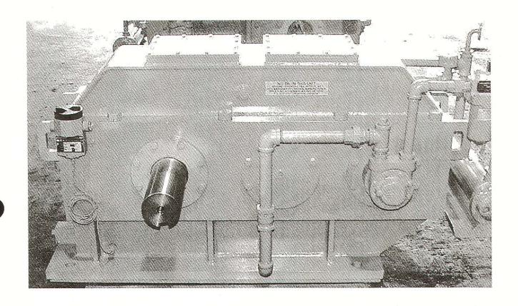
Shaft Driven Pump uses rotating shaft end to drive mechanical pump.
