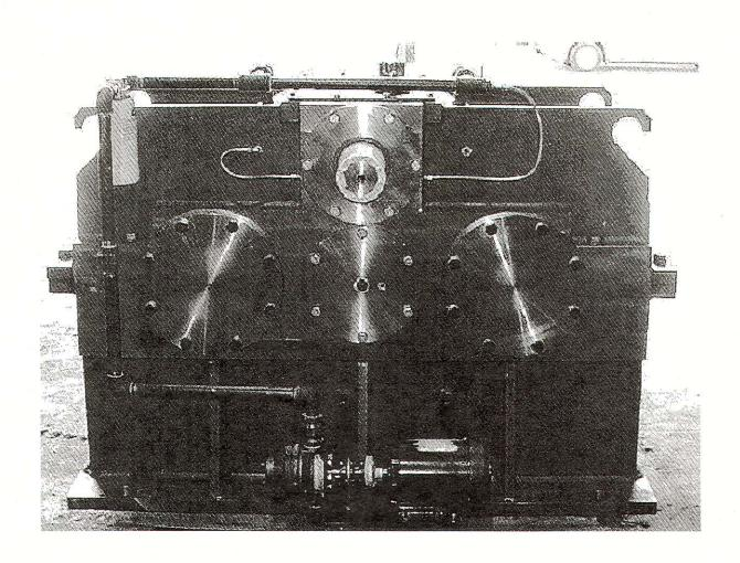
Motorized Pump uses electric motor driven pump to supply oil to strategic points.
