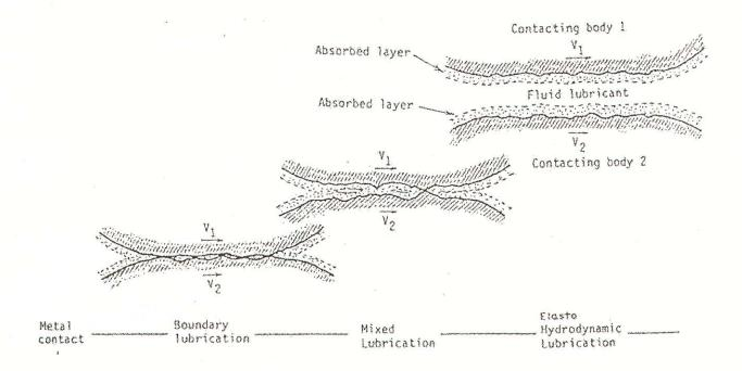
REGIME 1: Boundary lubrication exists where the gears are wetted with oil but the film thickness developed is small compared to the tooth surface associated with gears operating at low pitch line velocities and/or heavy loads.
