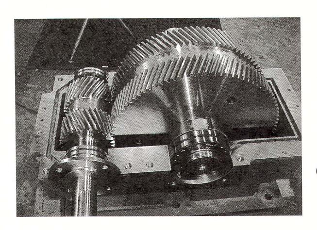
Splash relies on centrifugal force to sling oil inside housing.
