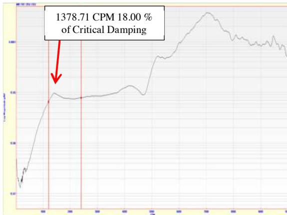
**Figure 28. ID Fan A, OB Pedestal FRF Reference DOF 135X:135X.**
