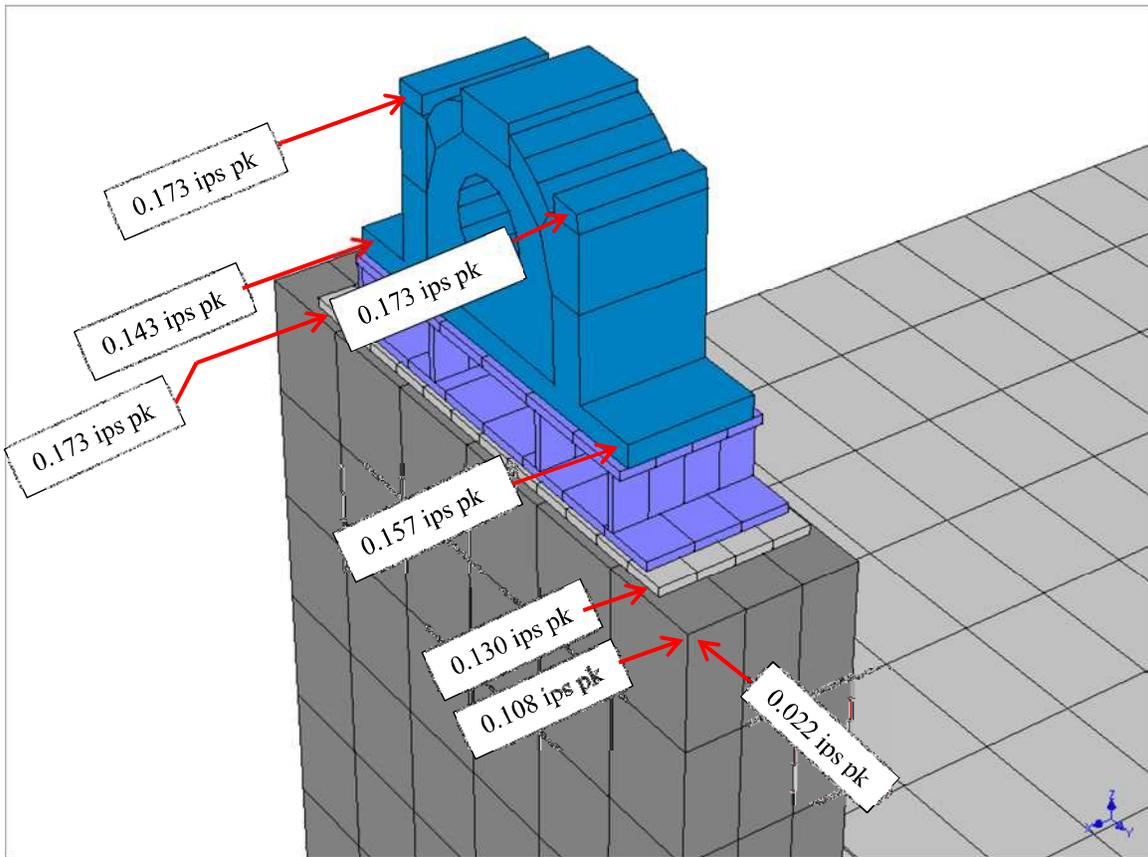
**Figure 24 ID Fan A OB Bearing & Pedestal With Some DOF Vibration Amplitude Labeled at 2X Run Speed.**
