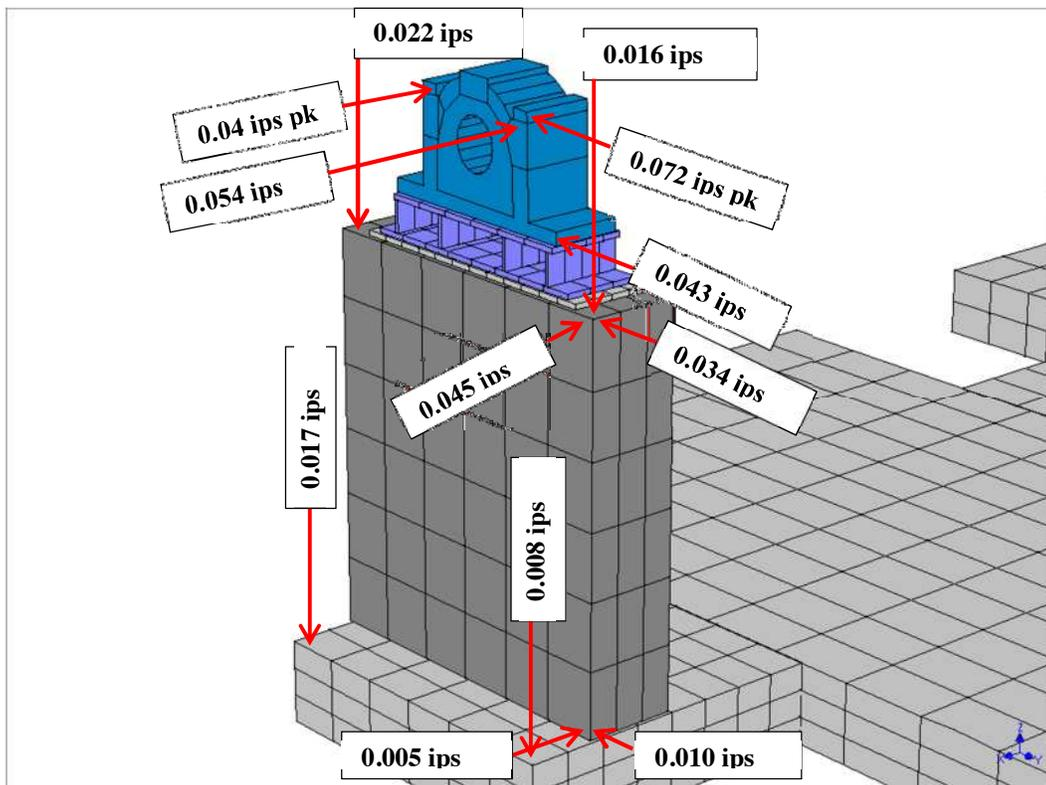
**Figure 20. ID Fan A OB Pedestal Vibration at 1X Run Speed Frequency.**
