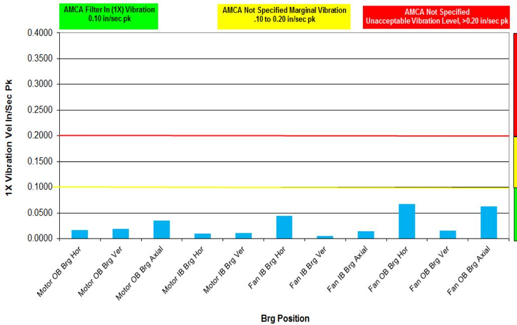
Figure 10. ID Fan A, 1X Vibration in/sec pk.
