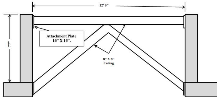
**Figure 2. Brace of 8" Square Tubing Bolted to ID Fan Outboard Bearing Concrete Pedestals.**
