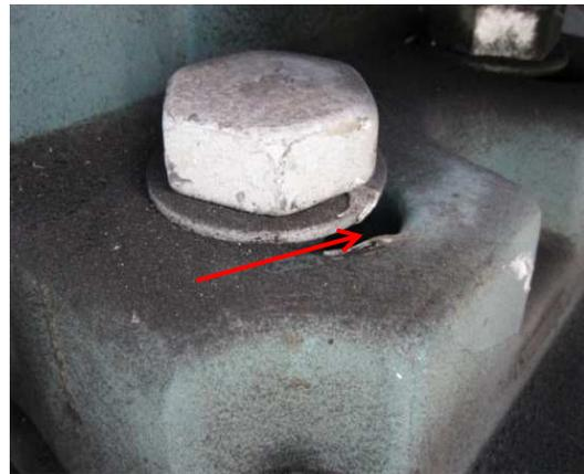
**Figure 7. ID Fan A, Inboard Bearing Housing Hold Down Bolt – Washer Was Too Thin.**
