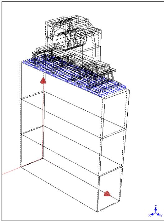
**Figure 32. ID Fan A Outboard Bearing Pedestal Modal Test, Mode Shape 2509 CPM Rocking Side-to-Side in Y.**
