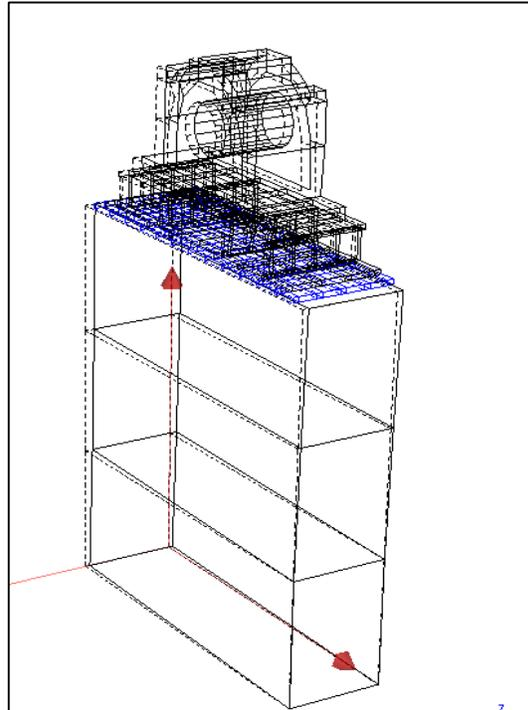
**Figure 34. ID Fan A Outboard Bearing Pedestal Modal Test Mode Shape 5107 CPM Rocking in X (Axial).**
