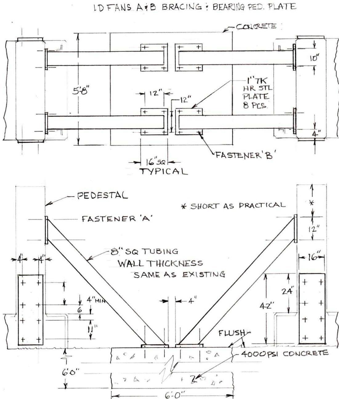
**Figure 36. ID Fans A & B Revised Bracing and Pedestal Plate Support.**
