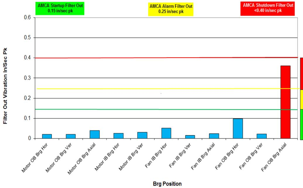
Figure 9. ID Fan A Overall Vibration (Filter Out) in/sec pk.
