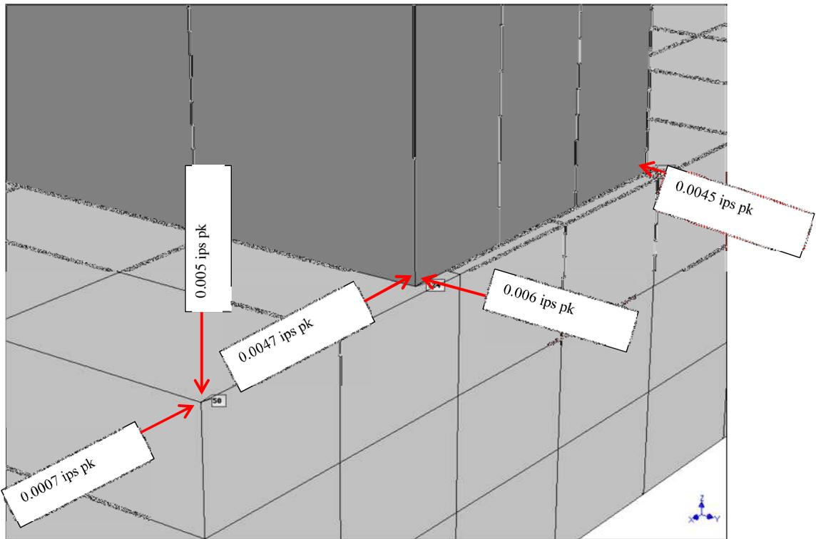
**Figure 25. ID Fan A, OB Bearing Pedestal Interface to Concrete Foundation.**
