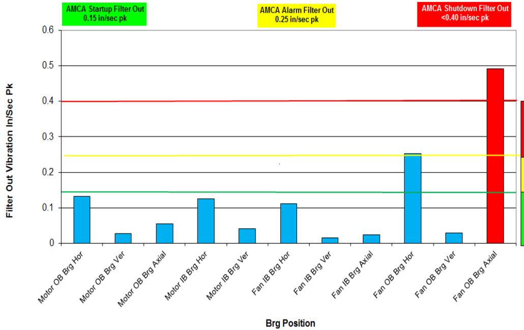
**Figure 13. ID Fan B, Overall Vibration in/sec pk.**
