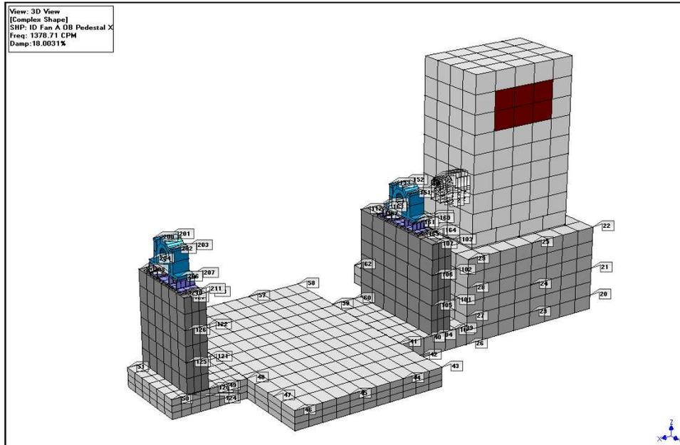
**Figure 16. ME’scopeVES Model of ID Fan A.**
