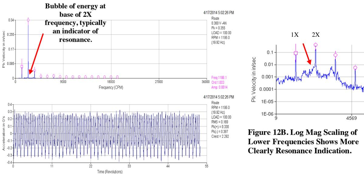
**Figure 12B. Log Mag Scaling of Lower Frequencies Shows More Clearly Resonance Indication.**
