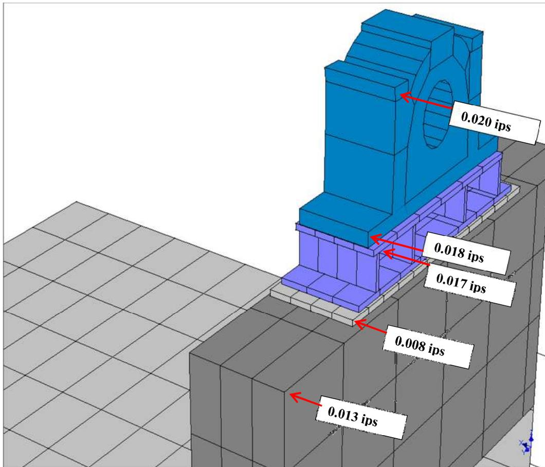
**Figure 22. ID Fan A, IB Brg Housing, Support and Pedestal. ODS Amplitude at 1X Shaft Rotational Frequency.**
