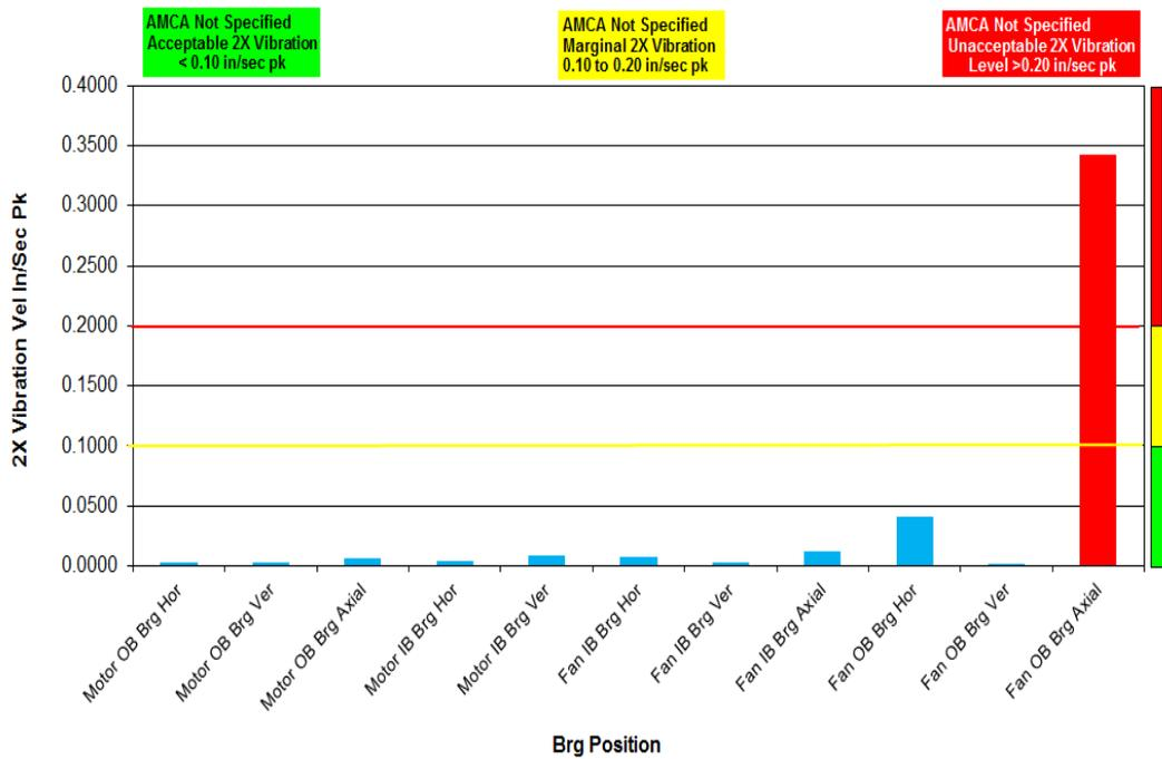
**Figure 11. ID Fan A, Bearing Housing 2X Vibration in/sec pk.**
