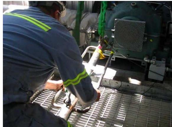
**Figure 29. ID Fan A, OB Bearing Pedestal Modal Test in X Direction (Axial). Impact Location was at base of the Bearing Housing since Concrete Pedestal Was Not Accessible.**
