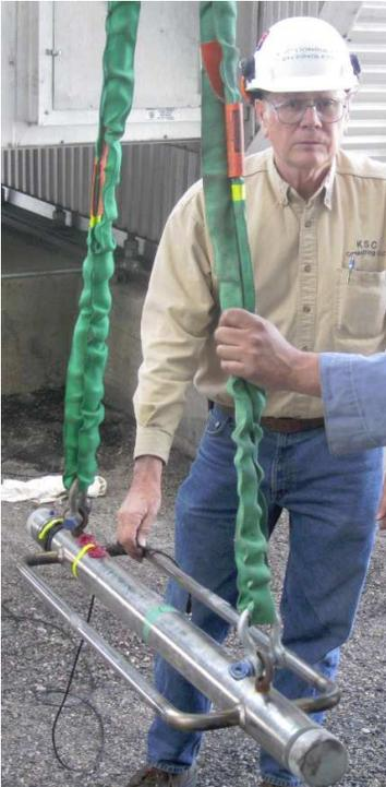
**Figure 26. Author (Singleton) With Steel Ram Equipped With 50,000 lb<sub>f</sub> Force Head Supported by Nylon Slings.**
