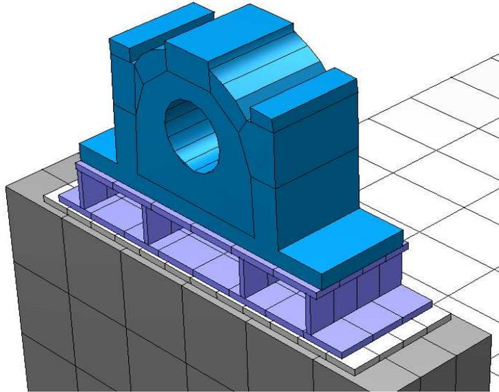
**Figure 17. Detail of Fan Outboard Bearing, Fabricated Base, Soleplate and Concrete Pedestal.**
