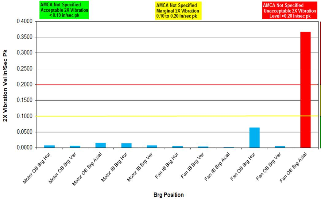
**Figure 15. Fan ID B, 2X Vibration in/sec pk.**
