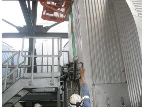
**Figure 27. ID Fan A, OB Bearing Pedestal. Modal Test in Y Direction (Side-to-Side).**
