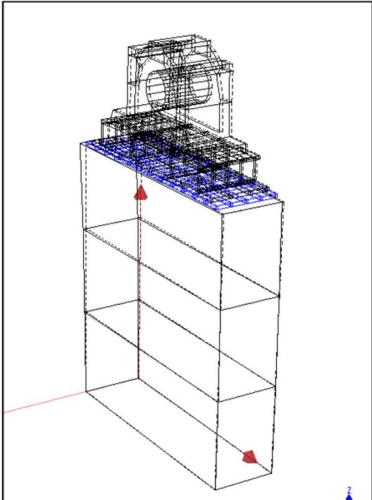
**Figure 33. ID Fan A Outboard Bearing Pedestal Modal Test, Mode Shape 1378 CPM Rocking in X (Axial).**
