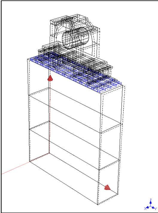
**Figure 31. ID Fan A Outboard Bearing Pedestal Modal Test, Mode Shape 1401 CPM Rocking Side-to-Side in Y.**
