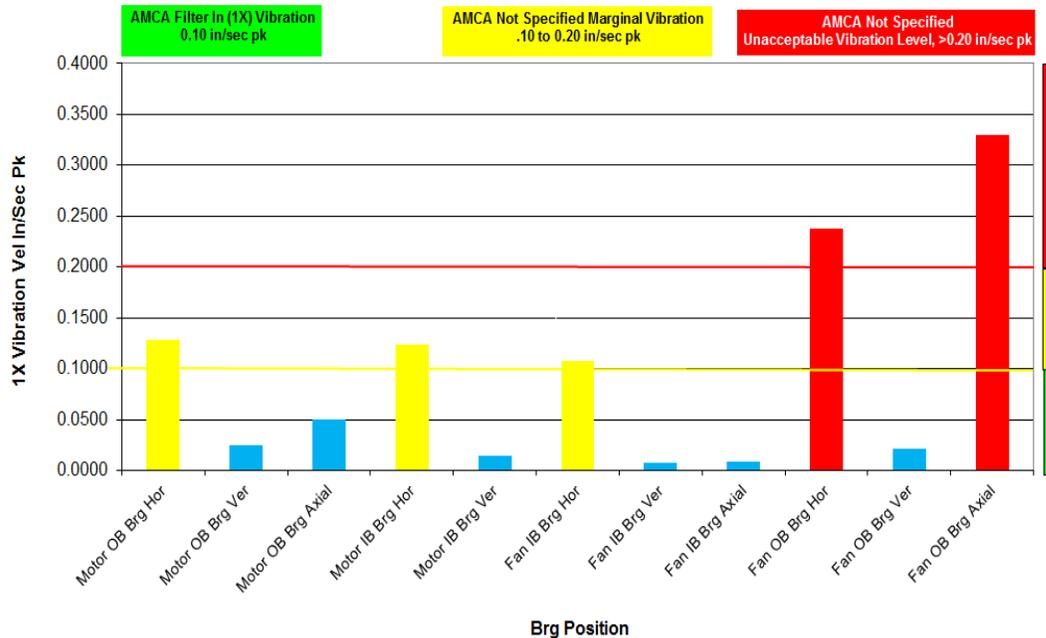
**Figure 14. ID Fan B, 1X Vibration in/sec pk.**
