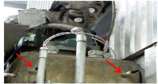
**Figure 19. Flat Rare Earth Magnets Attached 500mV/g Low Frequency Accelerometers.**
