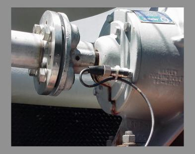
Coupling alignment is shaft alignment. If the shafts are aligned, the couplings will normally go along for the ride.
