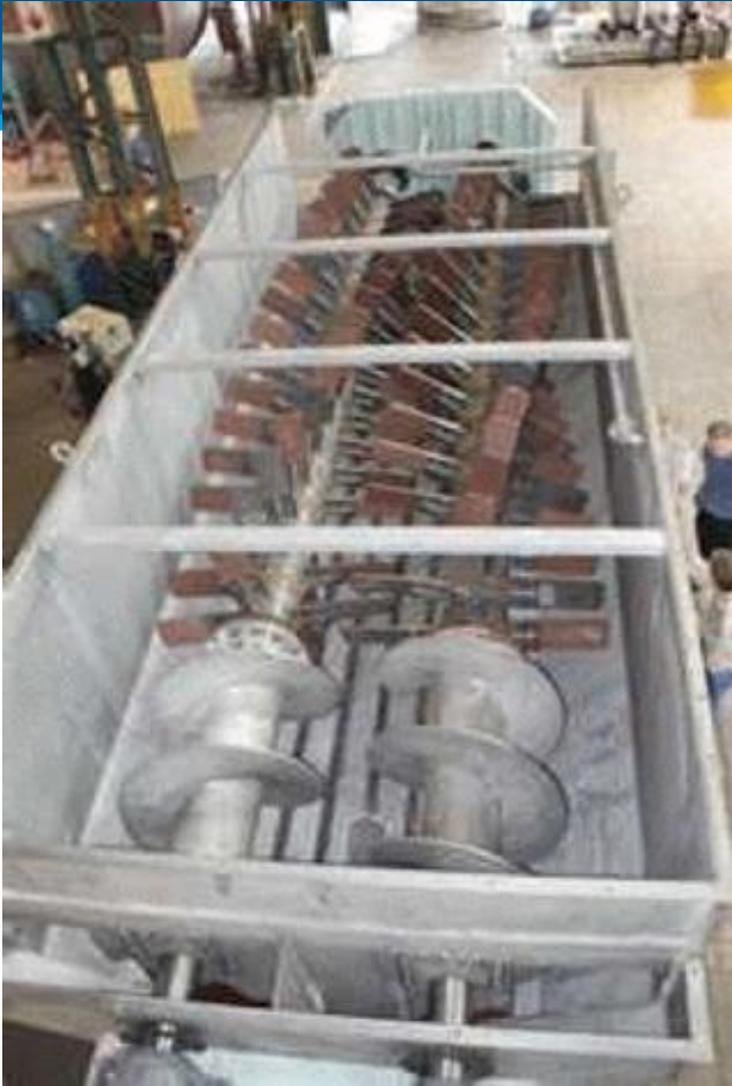
Solution: Stagger Paddle Arrangement (i.e. Controlling the Frequency & Magnitude of Dynamic Force)
