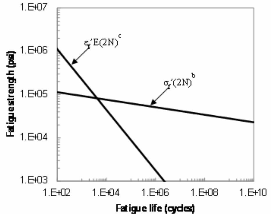
Fatigue life curves, developed from constant amplitude fatigue life tests, can be described by a low-cycle fatigue component and a high-cycle fatigue component. For high cycle fatigue,  $>1E06$  cycles, the equation simplifies to
