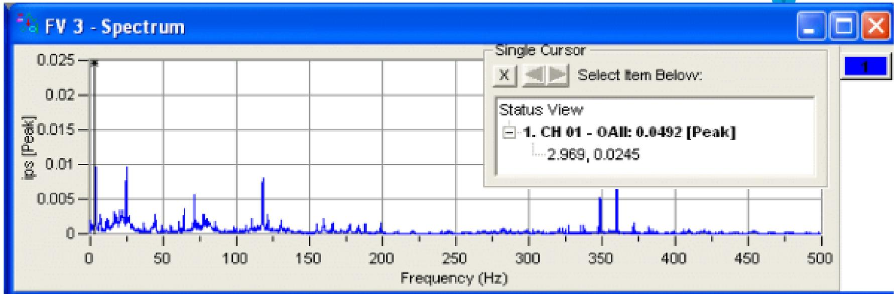
FFT of Motor Vibration (Horizontal) during normal mixing indicates low vibration level (0.025 ips) dominated by 4x Mixer Frequency (2.96 Hz).
