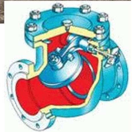
A check valve was provided in the discharge piping, close to the outlet of each pump, to isolate the pump from the header when it was not operating. At pump shutdown, the check-valve would slam shut when the flow reversed direction due to the positive pressure developed in the common header by the other operating pumps.
