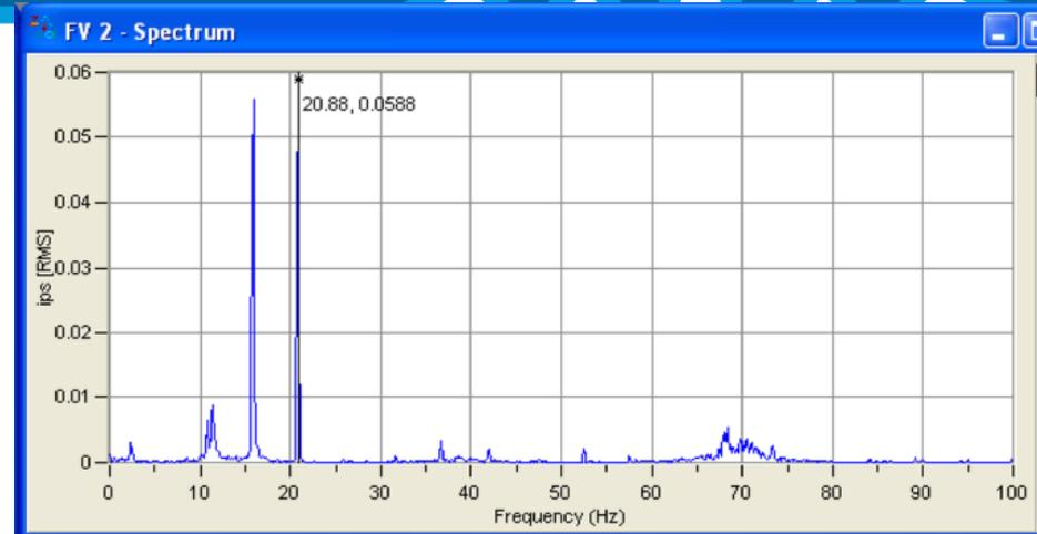
1800 rpm Pump Operates with VFD Control. At low flow (speed) settings, check valve not completely open. A rotating stall condition initiates. Vibration @ sub-harmonic frequency (~16 Hz) as well as operating speed (1250 rpm ~ 20.88 Hz).
