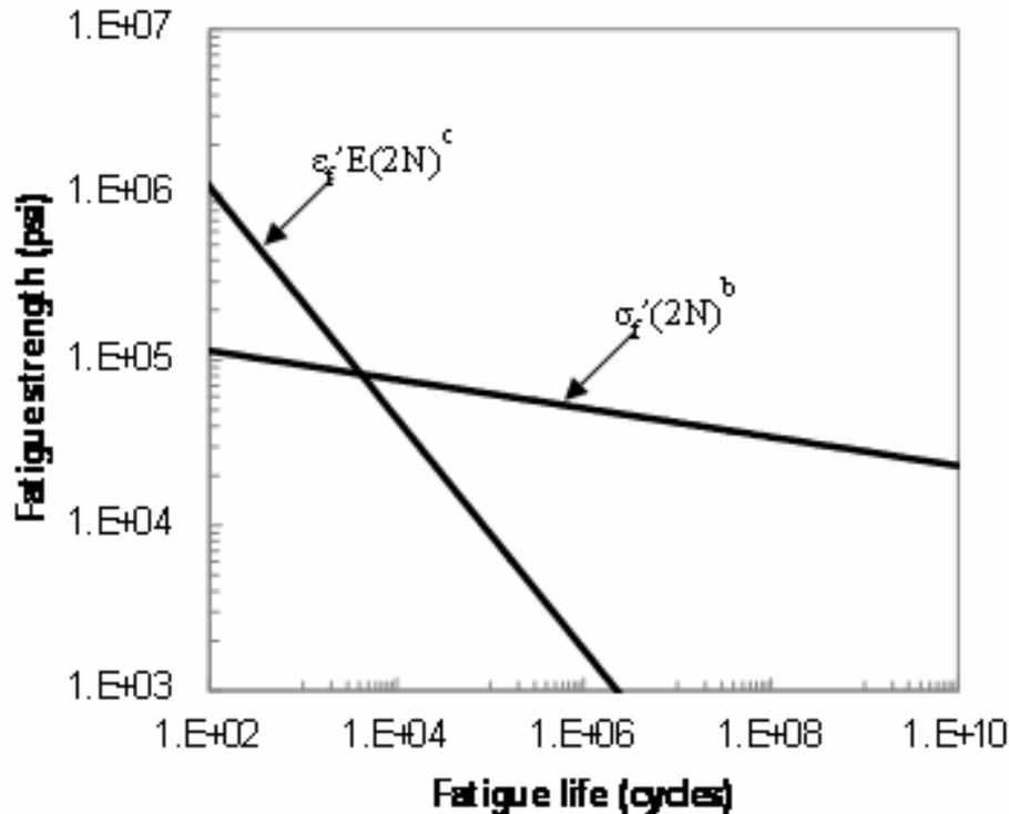
Note: Stress is measured or calculated @ point of max stress concentration. It is not the nominal stress
