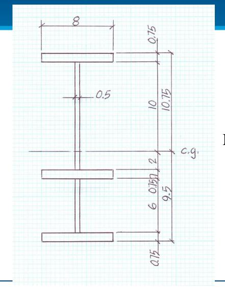
The Flange Stiffener Plates Resulted in a 2.60X increase in Stiffness K = 347,400/133,360 = 2.60Natural frequency only increased by 70.3/53.5 = 1.31x.
