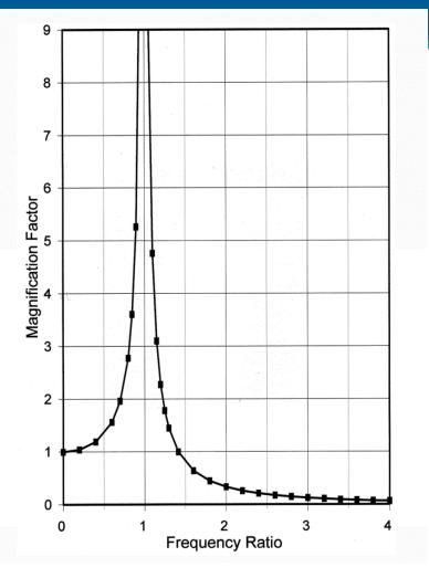
$AF = 1/[\{1 - (f_d/f_n)^2\}^2 + (2\zeta f_d/f_n)^2]^{1/2}$ Neglecting Damping:  $AF = 1/\{1-(f_d/f_n)^2\}^{1/2}$  $@ (f_d/f_n) > 1.414,$ Amplification Factor < 1.0Dynamic Force is attenuated instead of amplified. Objective:  $f_d >> f_n$
