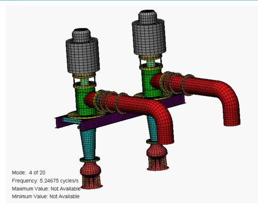
A flexible rubber spool piece was installed between the pump and check valve to minimize the mechanical transmission of dynamic force. After installation of the flexible spool piece, the maximum vibration level measured during a shutdown event was less than 1.0 ips, an order-ofmagnitude reduction from the original configuration.
