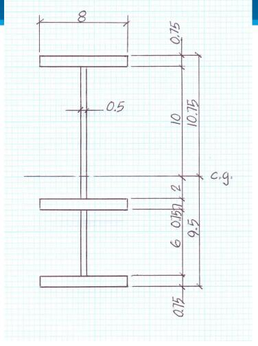
As Beam is stiffened, hysteretic damping (due to strain) is lowered. The damping factor ( $\zeta$ ) may be 0.03 for the original beam and 0.026 for the modified beam.
