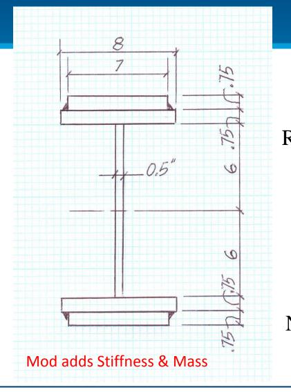
The Flange Stiffener Plates Resulted in a 1.95X increase in Stiffness k = 260,880/133,360 = 1.95Natural frequency only increased by 59.4/53.5 = 1.11x.
