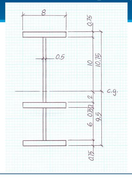
$k = 48 EI/L^3 =$  $48(29,000,000)(1455.5)/(180)^3 =$ 347,400 lb/in A = (.75)(8) + (.50)(6) + 18 = $27.0 \text{ in}^2$ m = 27.0(180)(0.283)/386.4 =3.56 lb-sec<sup>2</sup>/in m/2 = 1.78 lb-sec<sup>2</sup>/in  $f_n = (1/2\pi)[347,400/1.78]^{1/2} =$ 70.3Hz vs 53.5 Hz Vibration Institute
