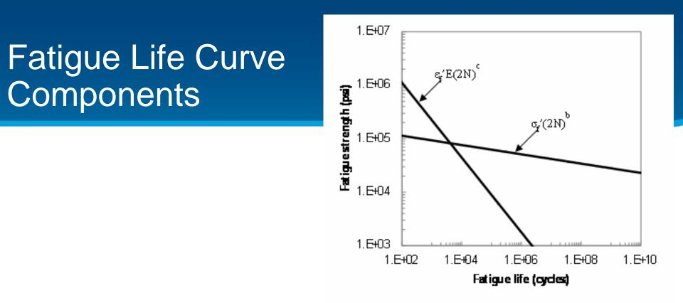
Fatigue life curves, developed from constant amplitude fatigue life tests, can be described by a low-cycle fatigue component and a high-cycle fatigue component. For high cycle fatigue,>1E06 cycles, the equation simplifies to
