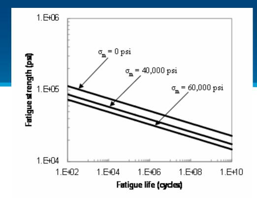
Both fan wheels are constructed of same material and operate under a continual mean stress of 40,000 psi. The high-cycle fatigue life equation for this material is defined by:
