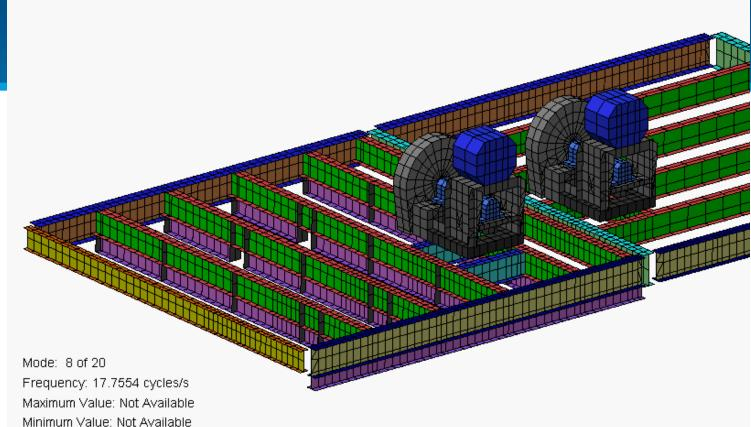
Natural Freq of Modified Floor = 17.75 Hz Freq Ratio =14.83/17.75 = 0.835
