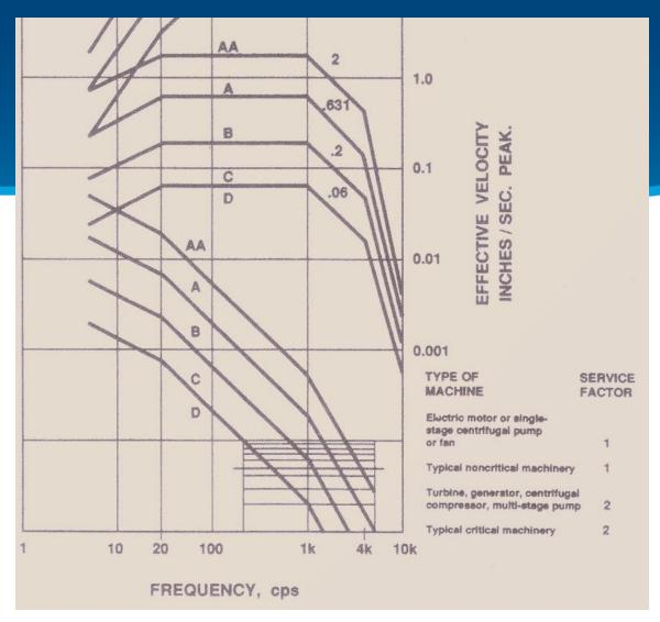
A Line @ 5 Hz; V < 0.30 ips; Critical Equipment has Service Factor = 2 A Line @ 20 Hz – 1 kHz; V < 0.63 ips
