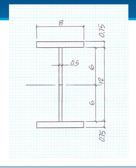
$k = 48 EI/L^3 =$  $k = 48(29,000,000)(560)/(180)^3 =$ 133,660 lb/in  $A = 2(.75)(8) + (.50)(12) = 18 \text{ in}^2$ m = 18(180)(0.283)/386.4 =2.37 lb-sec<sup>2</sup>/in  $m/2 = 1.185 \text{ lb-sec}^2/\text{in}$  $f_n = (1/2\pi)[133,660/1.185]^{1/2} =$ 53.5 Hz
