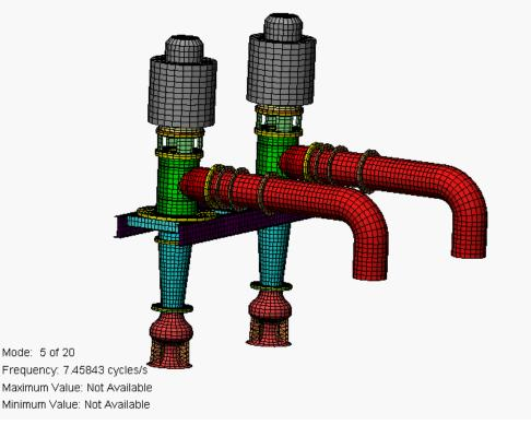
Mode Shape for Natural Frequency excited by Impulse Force created by Check Valve.
