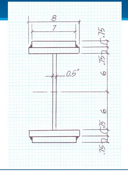
$k = 48 EI/L^3 =$  $k = 48(29,000,000)(1093)/(180)^3 =$ 260,880 lb/in  $A = 2(.75)(7) + 18 = 28.5 \text{ in}^2$ m = 28.5(180)(0.283)/386.4 =3.75 lb-sec<sup>2</sup>/in  $m/2 = 1.875 \text{ lb-sec}^2/\text{in}$  $f_n = (1/2\pi)[260,880/1.875]^{1/2} =$ 59.4 Hz vs 53.5 Hz
