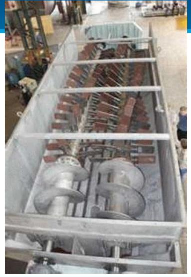
Solution: Stagger Paddle Arrangement (i.e. Controlling the Frequency & Magnitude of Dynamic Force)
