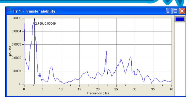
Natural Frequency Test of Motor Support Structure identifies fn ~ 2.7 Hz.
