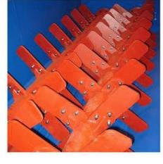
Problem: The rotating speed of the paddle rotor was 65 rpm (1.08 Hz). Each row of paddles contained four paddles and all paddles were in line from front to back of the machine, the log washer produced pulsations 4 times per revolution of the rotor which was  $4 \times 1.08 \sim 4.3$  Hz. This matched natural frequency of bldg and led to plant shutdown.
