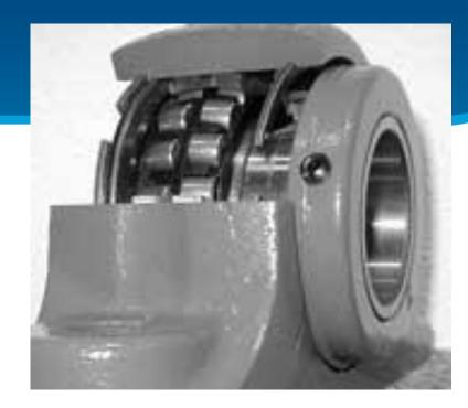
The American Bearing Manufacturers Association (ABMA), defines the Basic Rating Life, L10 as the bearing life associated with a 90% reliability when operating under conventional conditions.
