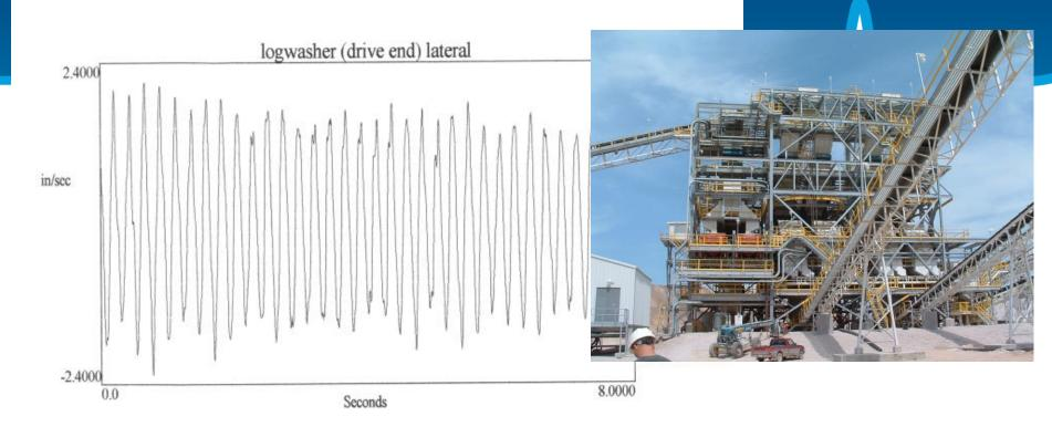
Structural vibration was dominated by response at 4.3 Hz, reaching magnitudes of 2.4 ips with the machine only lightly loaded. Peak-Peak Displace =  $2x2.4/2\pi(4.3) \sim 180$  mils @ Machine Peak-Peak Displace > 0.6 inches @ top of bldg
