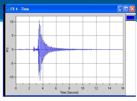
A check valve was provided in the discharge piping, close to the outlet of each pump, to isolate the pump from the header when it was not operating. At pump shutdown, the check-valve would slam shut when the flow reversed direction due to the positive pressure developed in the common header by the other operating pumps.
