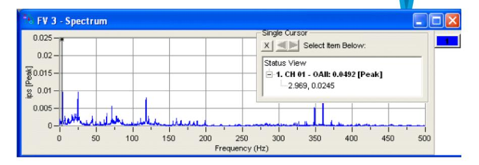
FFT of Motor Vibration (Horizontal) during normal mixing indicates low vibration level (0.025 ips) dominated by 4x Mixer Frequency (2.96 Hz).
