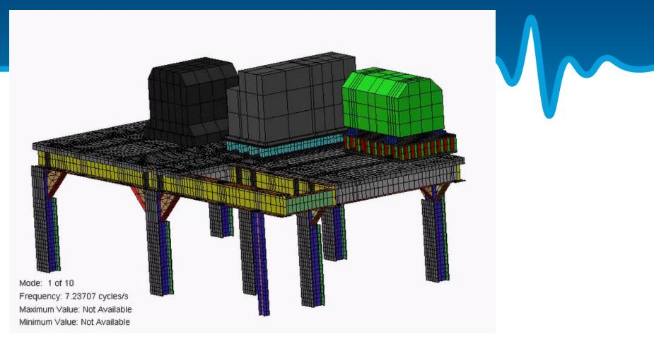
Natural Frequency increases to 7.3 Hz Close to Objective
