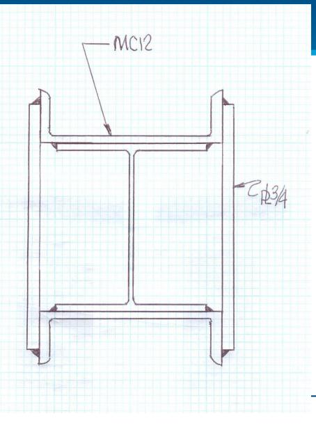
**FEA Freq Ratio:** 7.3/2.7 = 2.7x Increase  $I_{\text{original}} = 107 \text{ in}^4$  $I_{\text{modified}} = 1435 \text{ in}^4$ Stiffness Increase = 13.6x**Projected Nat Freq Increase:**  $(13.6)^{1/2}(2.7) = 9.96 \text{ Hz} >$ FEA Calculation of 7.3 Hz
