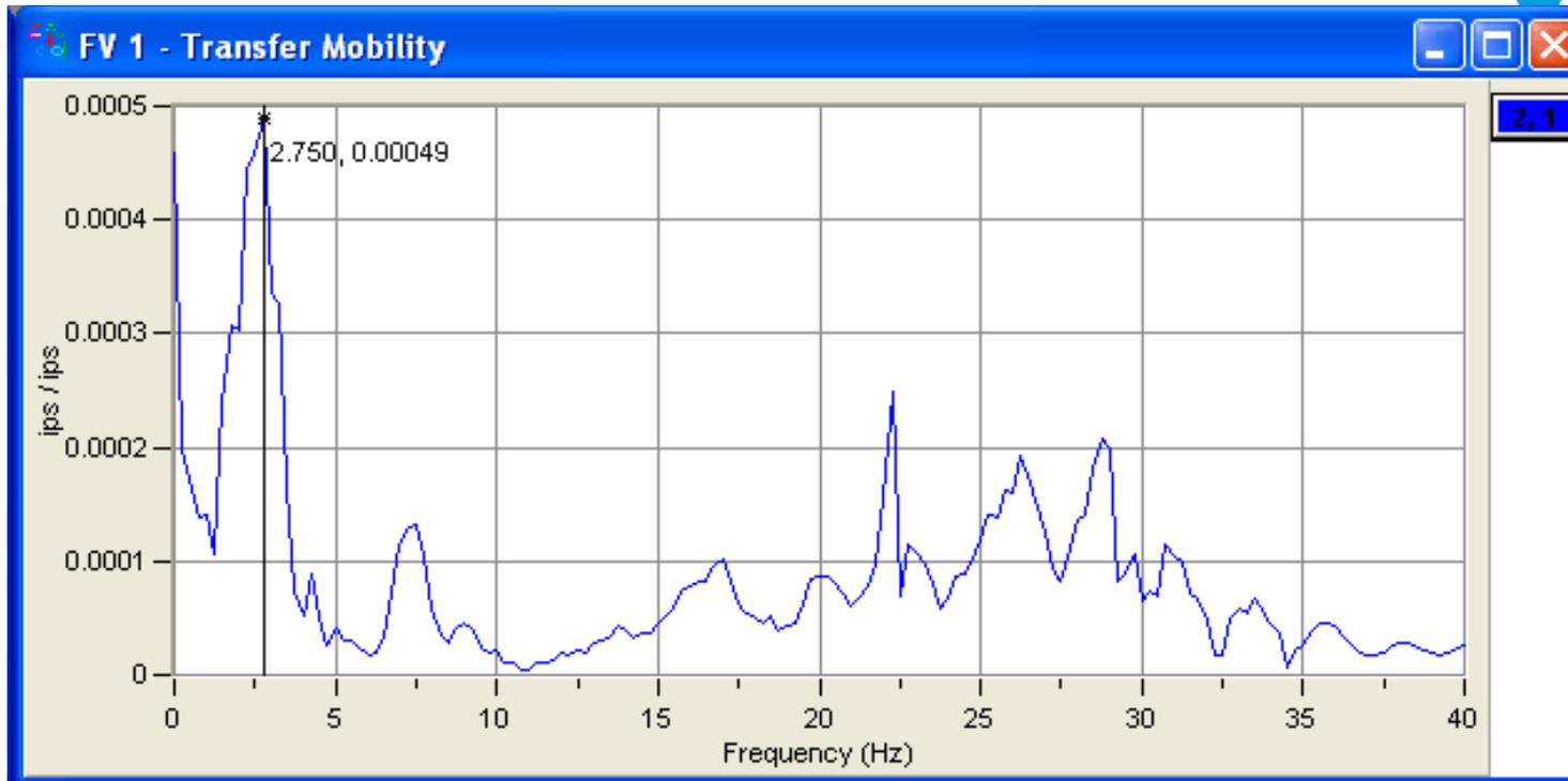
Natural Frequency Test of Motor Support Structure identifies  $f_n \sim 2.7$  Hz.
