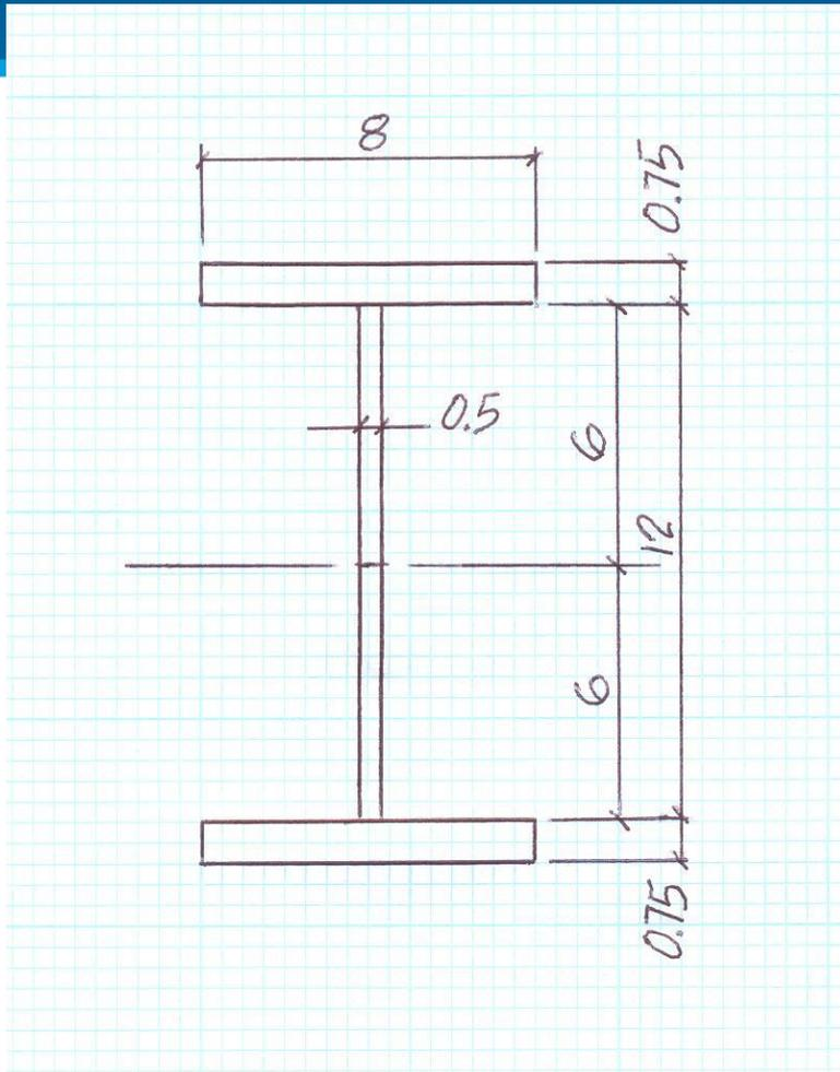
$$\text{Flexural Stiffness} = k = \frac{48EI}{L^3}$$
