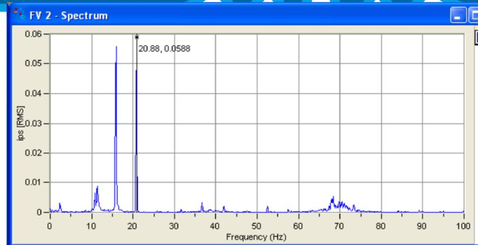
1800 rpm Pump Operates with VFD Control. At low flow (speed) settings, check valve not completely open. A rotating stall condition initiates. Vibration @ sub-harmonic frequency ( $\sim 16$  Hz) as well as operating speed (1250 rpm  $\sim 20.88$  Hz).
