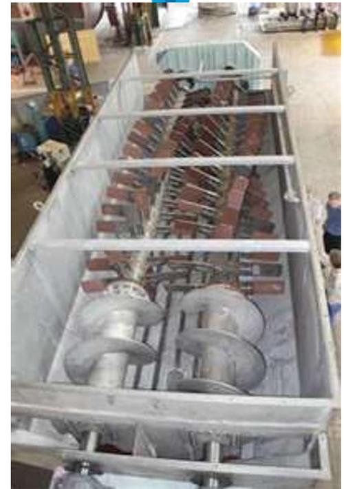
Problem: The rotating speed of the paddle rotor was 65 rpm (1.08 Hz). Each row of paddles contained four paddles and all paddles were in line from front to back of the machine, the log washer produced pulsations 4 times per revolution of the rotor which was  $4 \times 1.08 \sim 4.3$  Hz. This matched natural frequency of bldg and led to plant shutdown.
