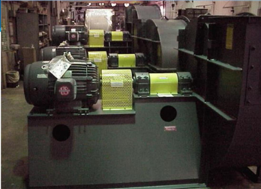
Consider a Fan that at one vibration level is subjected to 20,000 psi cyclic stress, with constant mean stress of 50,000psi, operating @ 1,200 rpm. (cycles =  $1.73E06$  per day)
