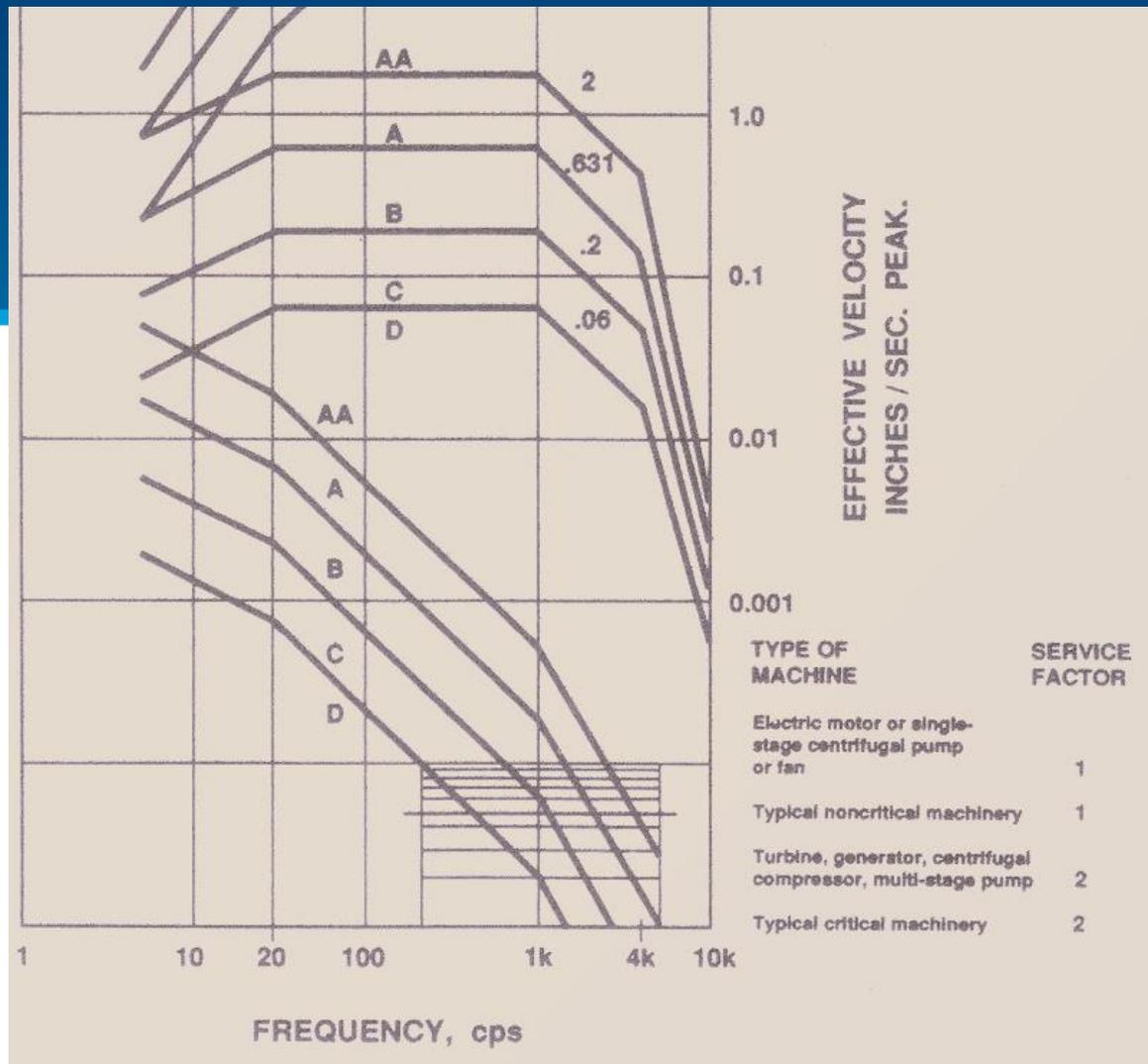
A Line @ 5 Hz;  $V < 0.30$  ips; Critical Equipment has Service Factor = 2
