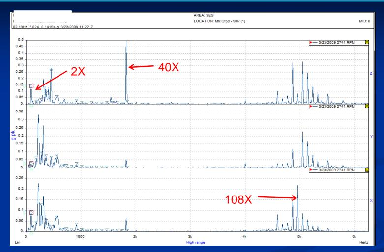
Here is the same high frequency data set in acceleration 108 side banded with 2X of running speed (i.e.) 2 x line frequency
