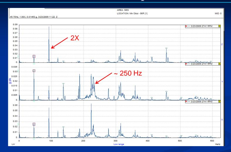
Here is the same data set with a low frequency span in acceleration
