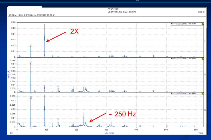
This is a data set from a VFD motor that has not had any routine problems just for review. Here is a low frequency span using velocity
