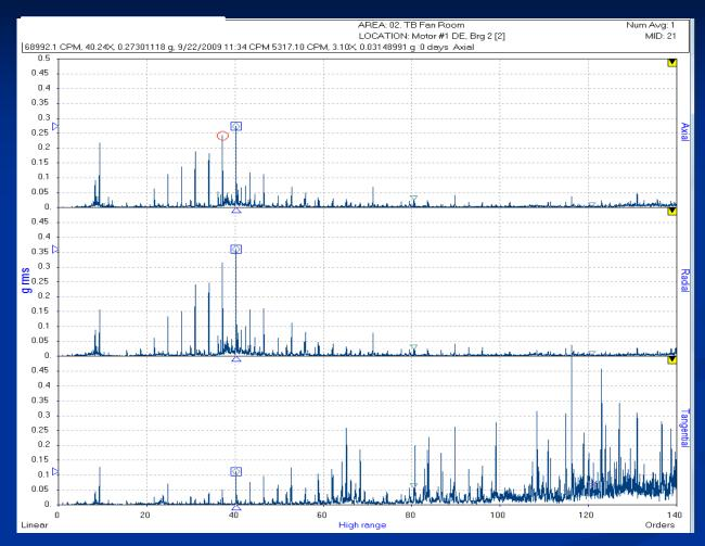
22 days later severe fluting in the bearing outer race. 09/22/09 – high freq - Driven End bearing
