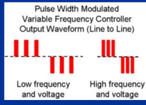
The PWM signal is then controlled to control the speed (i.e. the output) of the motor.
