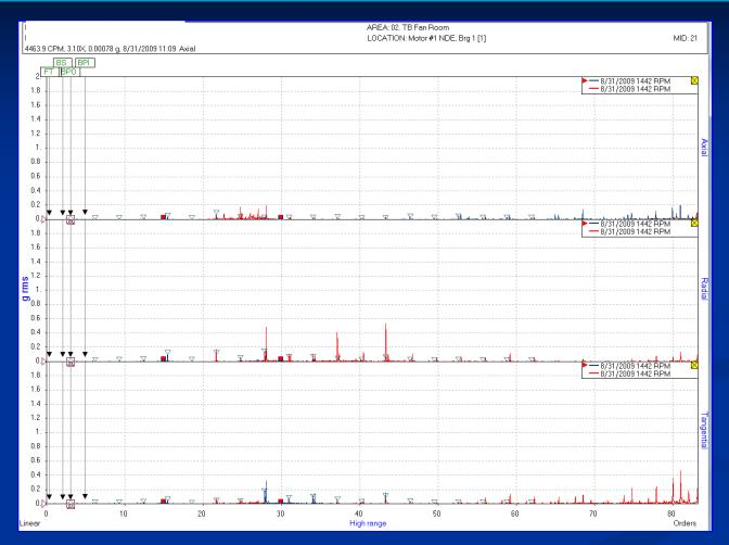
Here is a motor with what initially looked like a lack of lubrication during the initial data set. 8/31/09 – Low – high freq range
