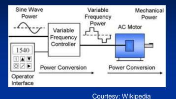
Typically, the power supply to the variable frequency controller will start out as 3-phase AC power. The AC signal will be rectified and converted to a DC signal.
