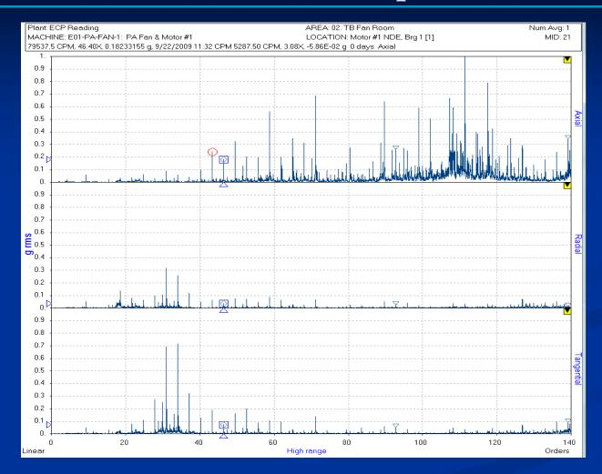
22 days later severe fluting in the bearing outer race. 09/22/09 – high freq - Non-Driven End bearing
