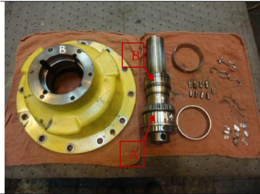
Fig 3. The high speed head components were disassembled, laid out and inspected. The bearing labeled B on the extended end of the shaft had failed. (043)
