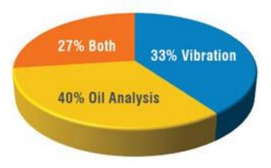
Bearing fault detection of early bearing failure (750 machines)
