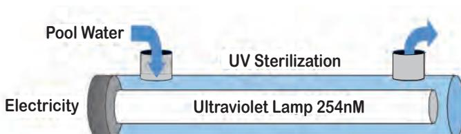
A properly designed, sized, and installed UV system will inactivate most micro-organisms passing through it very quickly. Because of this, UV has been hailed as an ideal solution for pool water sanitation.
