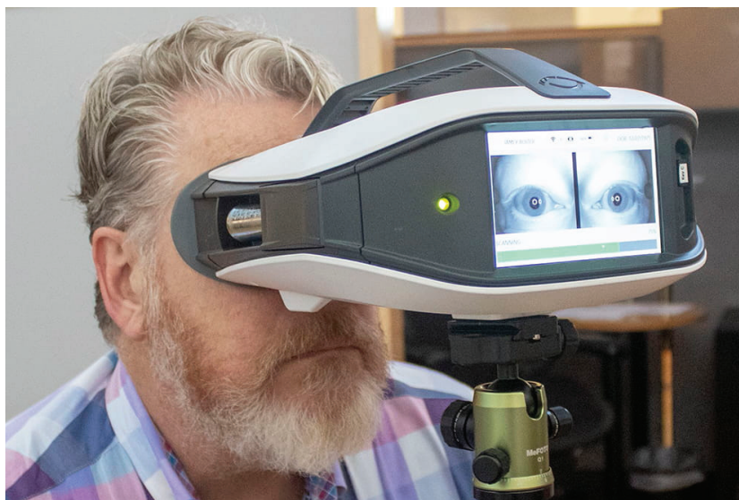
EyeStat delivers five light puffs of food-grade carbon dioxide at random intervals to the corner of the eyes over a 20-second time frame to assess the blink reflex. Photo courtesy of MUSC.
