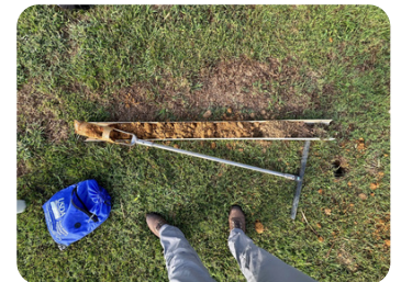
Manual auger and core sample taken by NRCS to test the type and health of the soil
