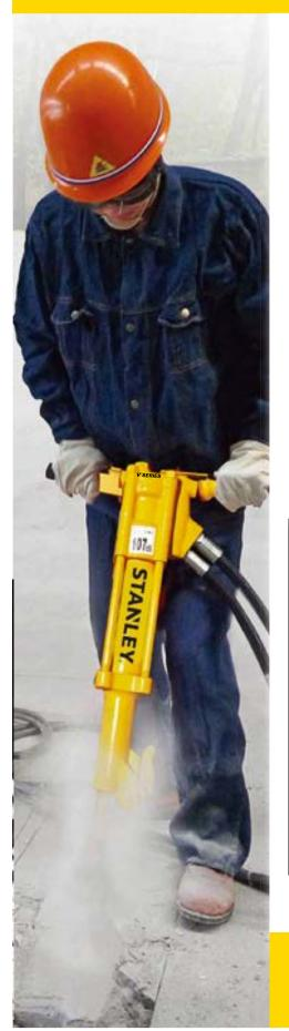
Professionals turn to hydraulic tools when they need to get the job done. Nothing matches the performance of hydraulic tools as compressed oil transfers energy more efficiently than compressed air. The inherent efficiencies result in longer life of the tool along with increased power and reliability.
