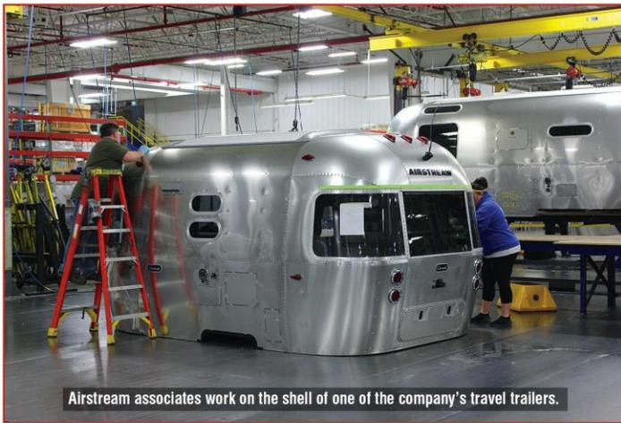
Airstream associates work on the shell of one of the company's travel trailers.
