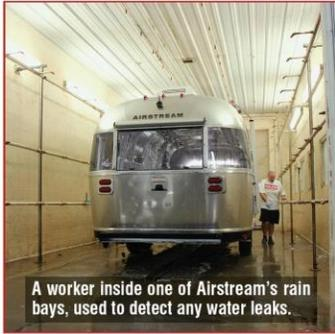
A worker inside one of Airstream's rain bays, used to detect any water leaks.
