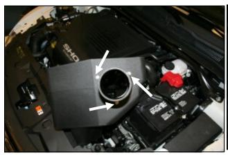
7. Install the Filter Adapter to the inside of the Cool Air 8. A) Install the Hump Hose, large side first (#4) onto 9. Remove the Air Temperature Sensor from the factory Box, CAB (#2) using the three 1/4"-20 hex head bolts the CAB tube. Loosely install the #56 Hose Clamp (#10) (#6) and 1/4" flat washers (#7) as shown.
