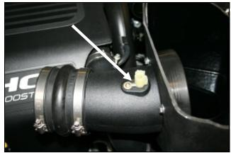
10. A) Transfer the factory Air Temperature Sensor into the Airaid Intake tube and align the sensor tab with the Groove in the tube. **B**) Secure the sensor to the tube using the 8-32 Button Head Bolt (#8) and the 3/4" washer (#9).
