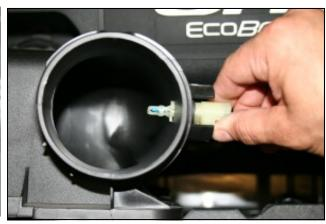
air box by rotating the sensor 1/4 turn counter clockwise and pulling outward.
