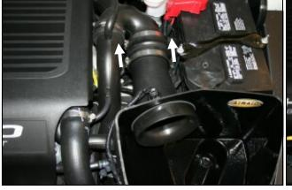
11. A.) Place the CAB in the original location of the Fac- 12. Install the Airaid Premium Filter (#1) onto the Filter tory Air box and secure using the factory hardware from adapter and tighten the clamp. step 4. B.) Slide the coupler and clamps onto 90 deg. Elbow pipe and tighten the clamps. C.) Reconnect the Air Temperature Sensor.
