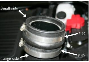
on the small side of the Hump Hose, and the #60 Hose Clamp (#11) on the Large side. ( B) Slide the Hump Hose and Clamps downward on the tube, creating a compact assembly as shown.
