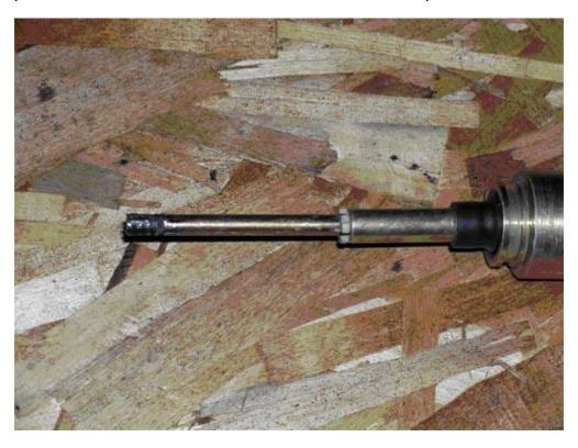
Slide the new cable end over the cable and measure to make sure you place the center of the hole in same location and rotation as the old black end. Once you are satisfied with the location, tighten down the set screw to lock it in place.
