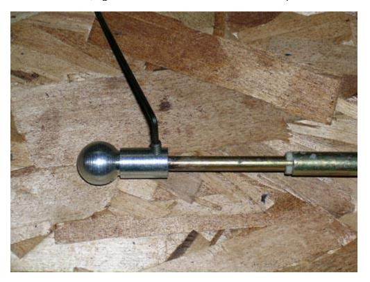
Here is what your new shifter cable looks like installed. (make sure you slide the wire clip through the holes and lock the clip around the ball.
