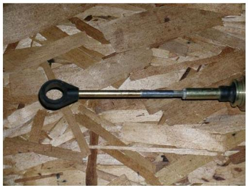
Remove the black plastic end the best way you can. Use a knife. Use a lighter to soften it (don't set your car on fire). Do not cut the metal rod; just remove the plastic. Here is how the shift cable looks without the plastic end.
