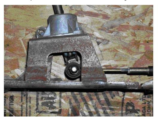
The first step is to measure the distance from the center of black plastic end to a reference point so can install the new end in the same location.
