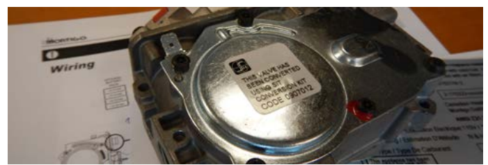
Figure 13.k Conversion label on valve
