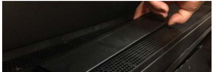
Figure 13.b Loosening the venturi
