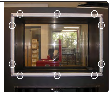
Figure 6.f Removing screws that secure screen.
