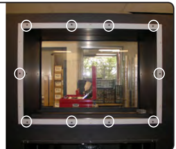
Figure 6.g Removing screws that secure screen.
