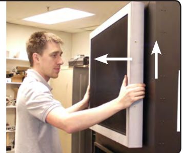
Figure 6.e Lifting screen frame up and out.
