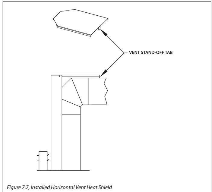
Figure 7.7, Installed Horizontal Vent Heat Shield
