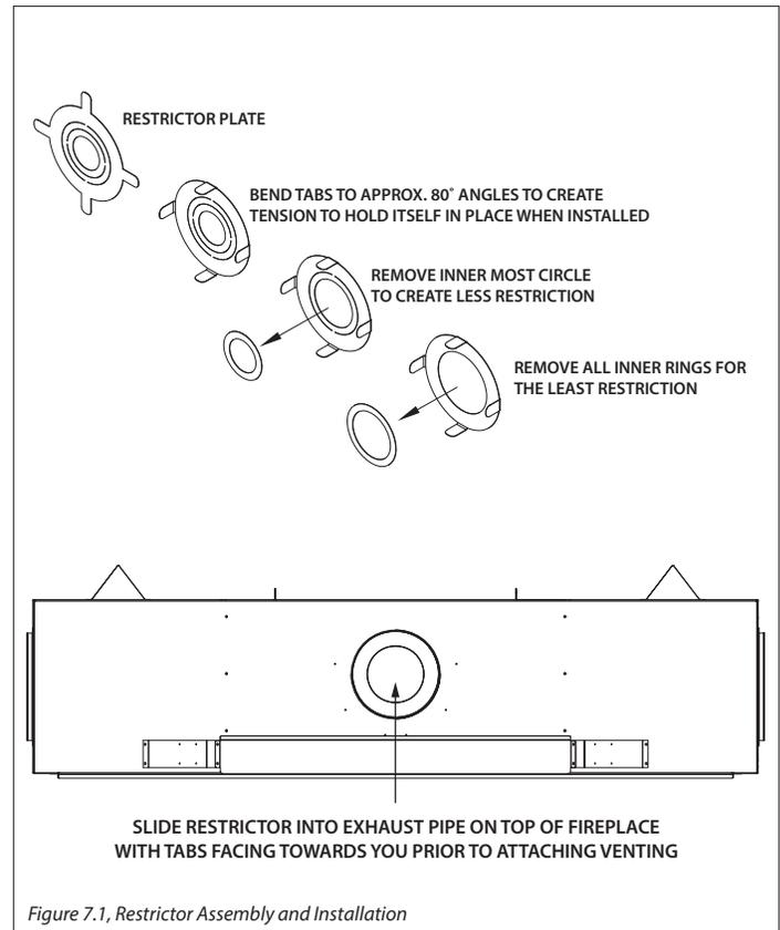
Figure 7.1, Restrictor Assembly and Installation
