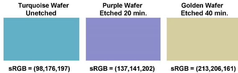
Fig. 2. Wafer colors and measured sRGB values.
