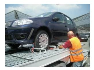
• Anchoring of motor vehicles located on tractor top and in last position on trailer top platform:
