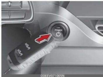
The side with the lock button should contact the POWER button directly.
