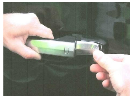
Figure 13: Key cylinder cover removal
