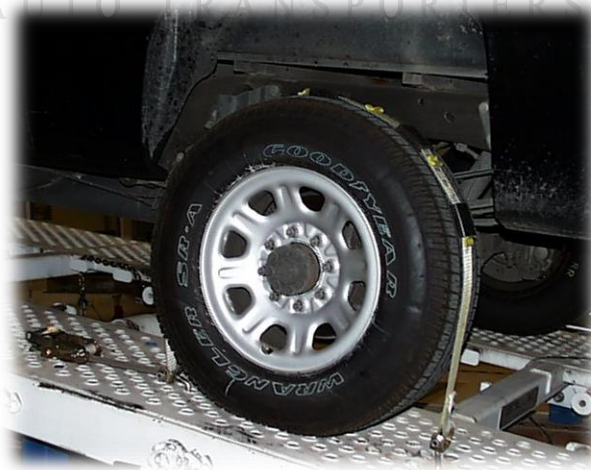
Figure 4: Haulaway soft-tie securement
