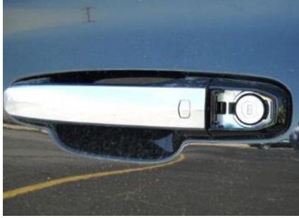
Figure 14: Key cylinder cover off
