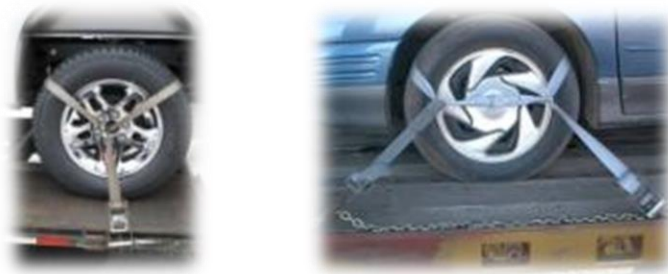
Figures 5 and 6: One point and two point soft-ties – NOT permitted
