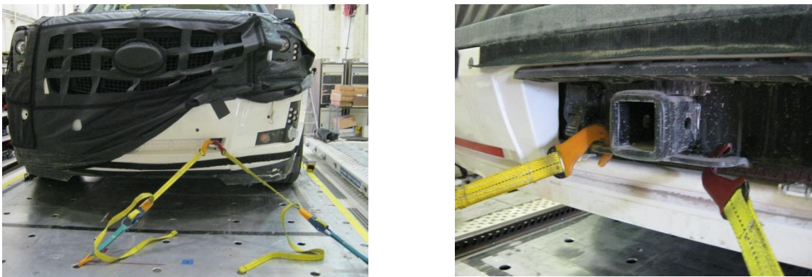
Figures 7 and 8: Front and rear Ocean lashings for Tahoe/Yukon
