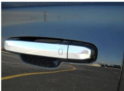
Figure 12: Key cylinder cover on
