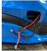
Pull both wires out of the opening to reveal both terminals. Connect the external power supply to the terminals (ensure you match the red positive cable to the red positive terminal and the black negative cable to the black negative terminal). Then, turn on the external power supply.
