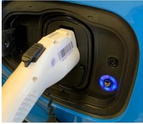
A solid blue segment represents 20% charge. A pulsating segment represents that portion of the battery is now being charged (active charging). If the
