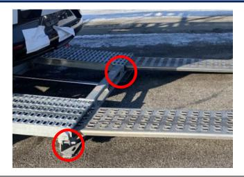
"Feet" must be deployed (see image above) to steady the deck as this heavy vehicle is loaded / offloaded to prevent the deck from bowing/curving which will lead to scraping of the lower front fascia or other types of damage to this vehicle. In the absence of "feet" or to provide extra support, place boards underneath the end of the deck.
