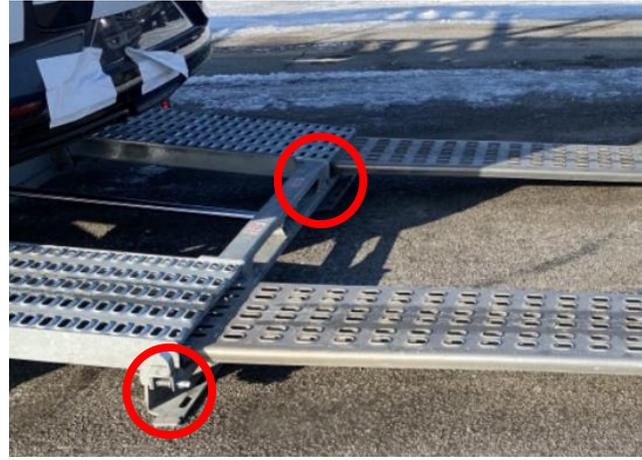
“Feet” must be deployed (see image above) to steady the deck as this heavy vehicle is loaded / offloaded to prevent the deck from bowing/curving which will lead to scraping of the lower front fascia or other types of damage to this vehicle. In the absence of “feet” or to provide extra support, place boards underneath the end of the deck.
