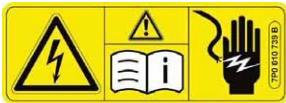
General warning notice on high voltage in engine compartment:
