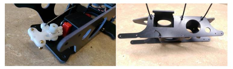
When building the chassis, you may want to assemble it first and then transfer parts. Install the rear first. Make sure to add spacers to the rear between the roll bar and gearbox, #4 washers work great If you are not using the roll bar, use the included black spacers. Zip ties are used to keep the side tabs located.
