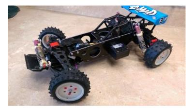
You can bolt the servo in place as original, or run the Team Associated bellcrank steering set part number 6255 included 3d printed bellcrank. We include a long 8-32 button head screw and nuts. The bellcrank is Associated part number 6281. Install as shown in the pic, if using stock tie rods choose the offset hole in the chassis.
