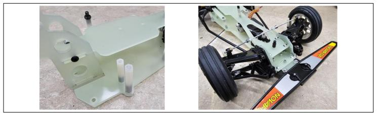
Step 10: Reinstall your front shock and transfer your steering servo. Replace the servo saver arm with part number 2 from the "P" parts tree. You will need to supply a linkage from the servo to the bellcrank, approx. 56mm from the center of each ball joint hole. Transfer the remainder of your electronics. Finally, check and set your toe. Enjoy!
