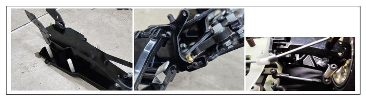
Step 8: Transfer your shock tower mount to the new upper plate using the included 3x8mm screws and plain nuts. Now reinstall the complete rear suspension using the stock self tapping screws for the shock tower, stock flanged nuts, and the included 3x30mm screws to go through the side plates and transmission. Use the included 3x12mm screws and locknuts to attach the lower plate to the lock plate and lower chassis.
