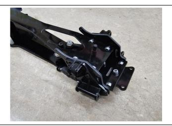
Step 6: Set the two rear side plates in place bridging the upper and lower chassis plates. Set the upper plate in place between the two side plates. Install the 3x8mm screws and nuts from the side plates to the upper chassis (not shown). This will help keep the assembly together for now. Install the lower lock plate using the 3x12mm screws and posts in the countersunk holes
