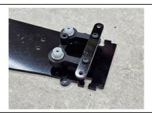
Step 2: Use the short flat head screws to bolt the two lower plates together with the 3mm locknuts.
