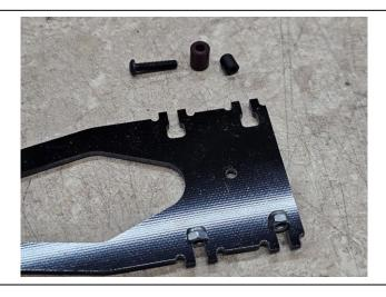
Step 5: Install the upper chassis to the chassis and right side assembly using 3x12mm screws. Now, assemble the left side to match what you have done on the right. If you will be using the rere sway bar, this is a great time to install it. With our chassis set it actually works quite well! Use the included spacers along with the stock collars to center the bar.
