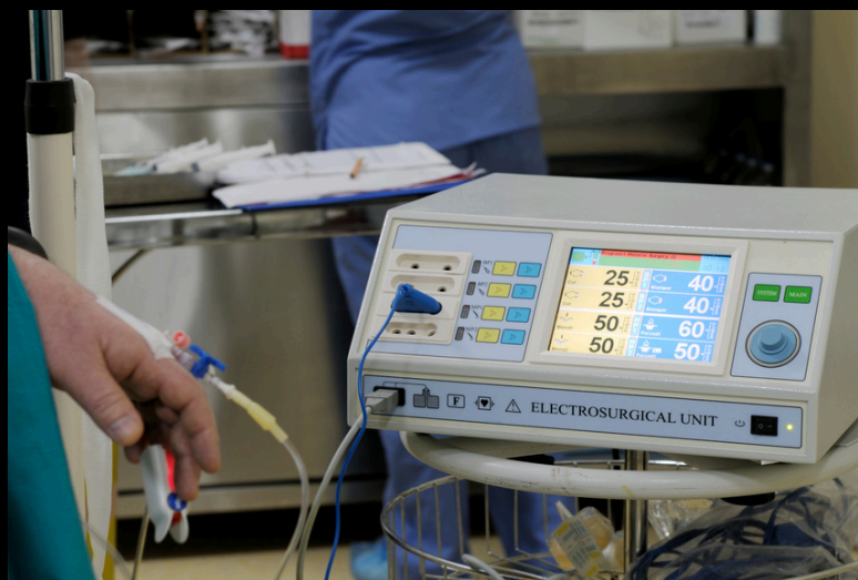
Picture of an Electrocautery unit (similar to what laser can do but uses Radio frequency that can cut and coagulate skin tissue)
