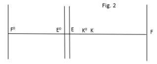
[Note 1 p10. The two points, which Moser (Repertorium der Physik, vol. V. p. 372) calls the first and second principal points of the eye, are essentially different from the main points introduced by Gauss and are identical to the so-called nodal points here.]
