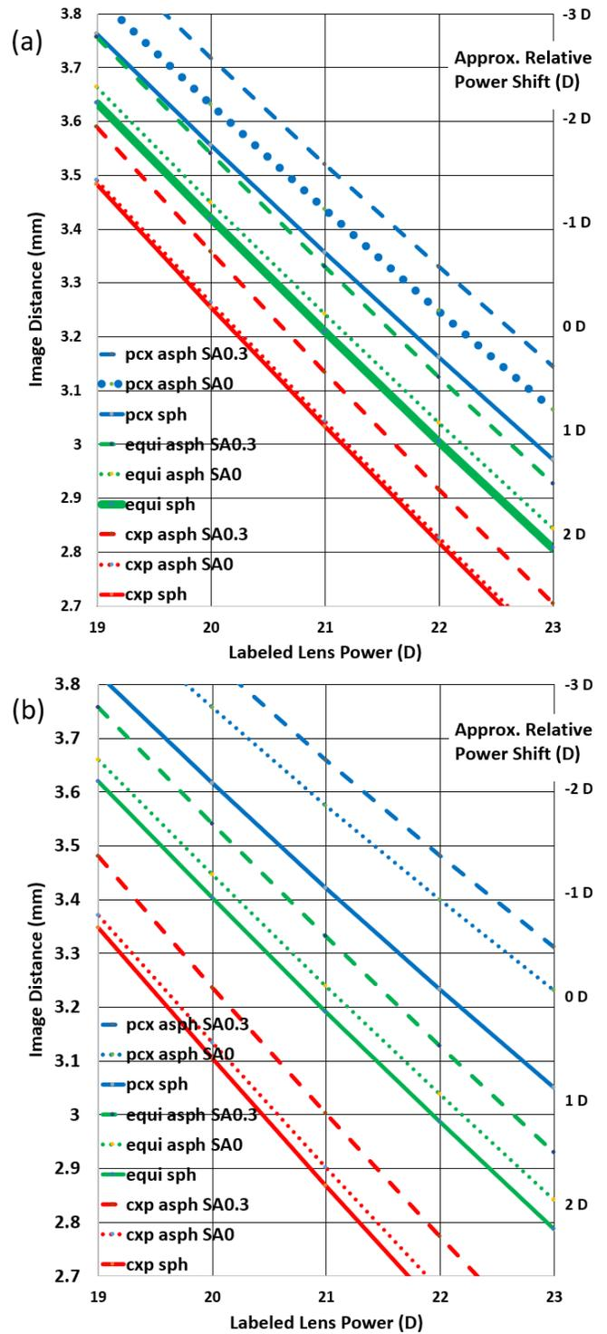
**Fig. 3.** Image distance values using the SA = 0 microns ISO2 model eye for refractive index values of (a) 1.55, and (b) 1.46. The approximate change in power value at the IOL is given at the right.
