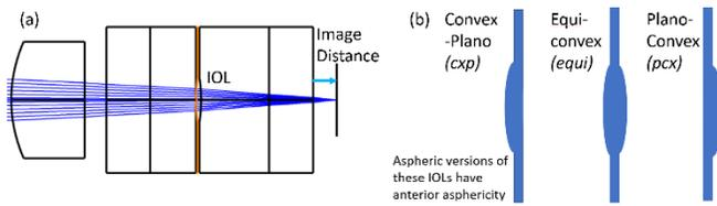
**Fig. 2.** (a) Image distances for the ISO2 model eye characterize A-Constant differences between lens styles. (b) Sketches of conceptual planar single-piece IOLs with three shape factors.
