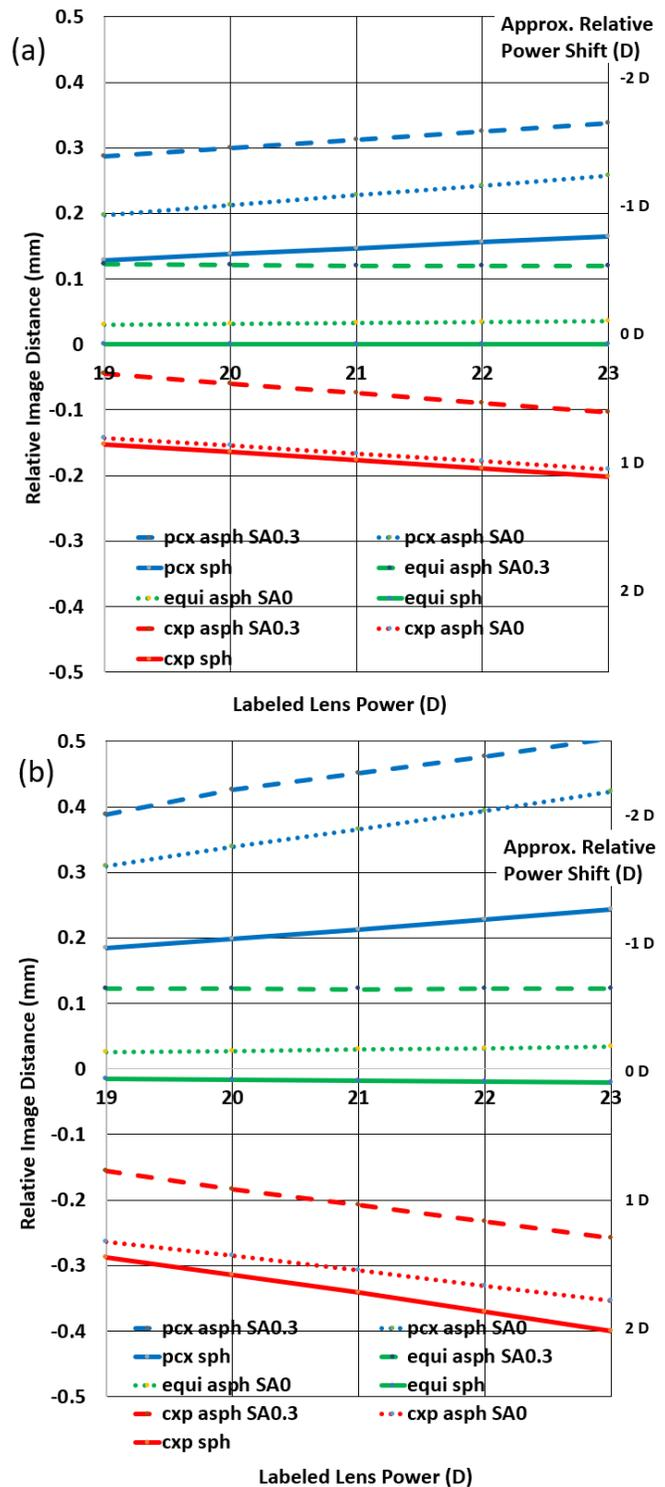
**Fig. 5.** Image distance values using the SA = 0 microns model eye with the value for the equi-biconvex IOL subtracted, for refractive index values of (a) 1.55, and (b) 1.46. The approximate power value change at the IOL is given at the right.
