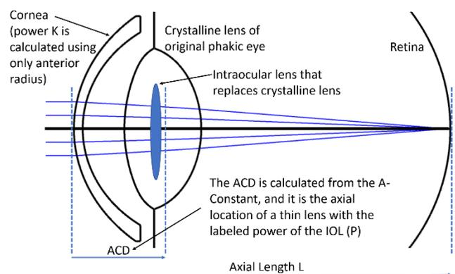
**Fig. 1.** Sketch of 0.7 mm thick IOL overlaid on an average phakic 70 year old eye with a 4.8 mm thick crystalline lens. A paraxial thin lens model for the eye is depicted by the vertical dotted lines. Only the ACD distance is unknown. An average value that is determined empirically from clinical data is used as an offset when calculating IOL powers for new patients.
