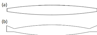
Fig. 5 Cross-sectional IOL profiles, with 6mm diameter, for (a) refractive index 1.55, and (b) refractive index 1.47 [18].
